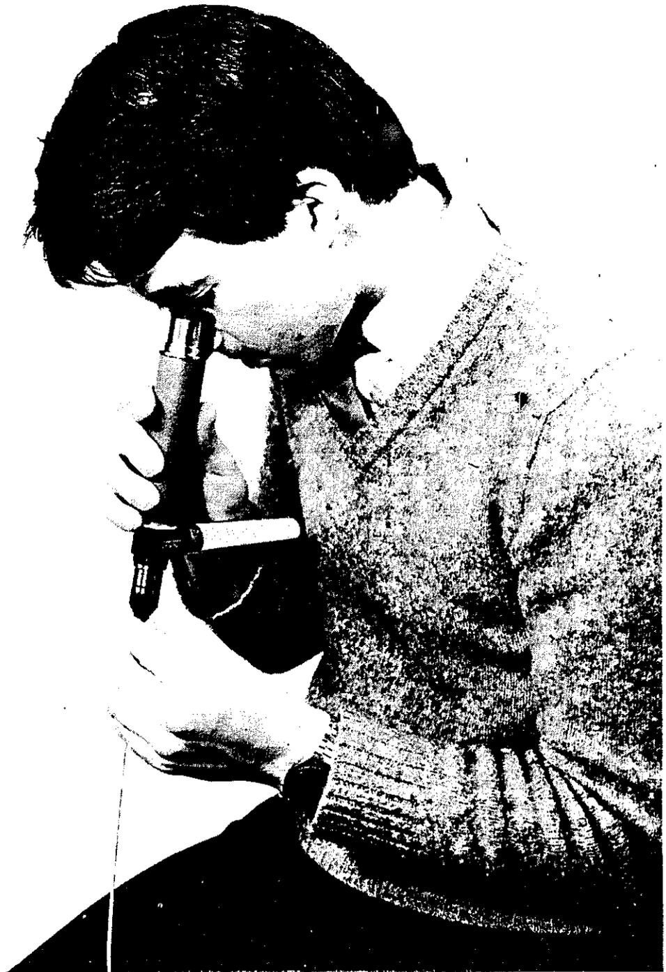
Figure 10. Visual Inspection of Cleaved Fibre End
