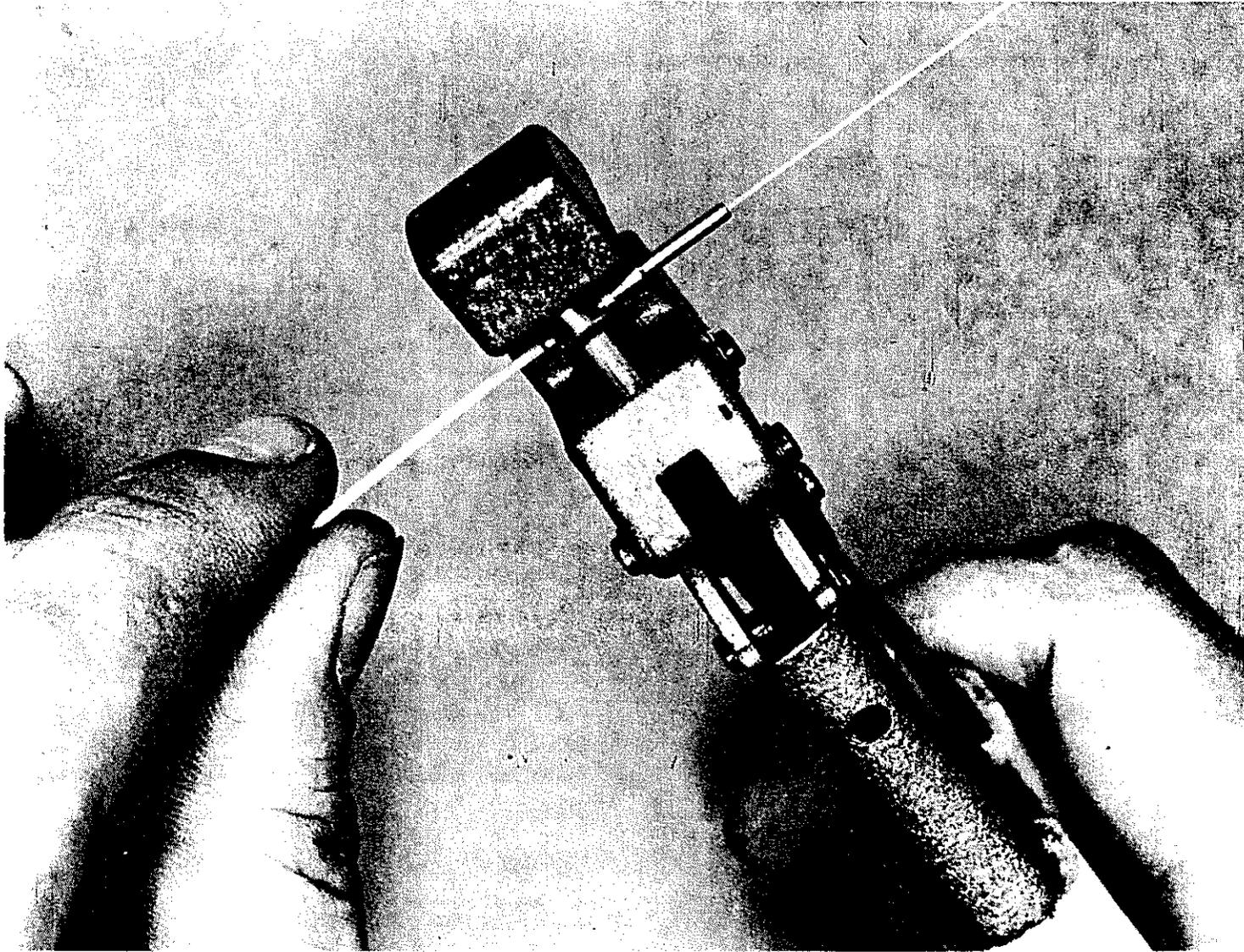
Figure 8. Crimping of Connector Alignment Ferrule
