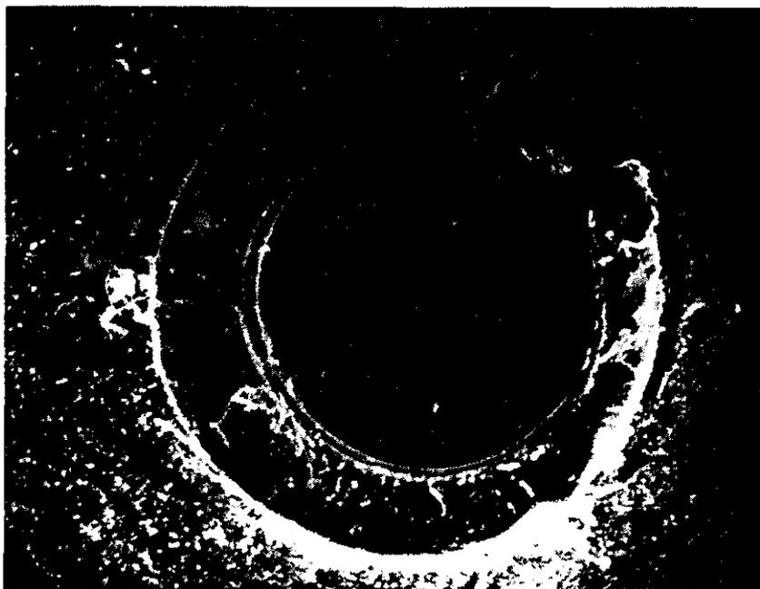
Figure 6. Cleaved Fibre Ends
