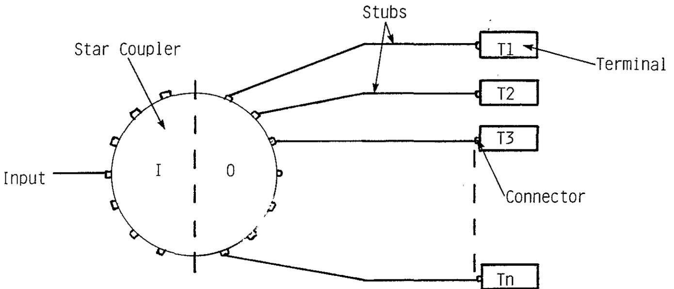
Coupling Ratio =  $\frac{1}{n} = 10 \log_{10} (1/n) \text{dB}$
