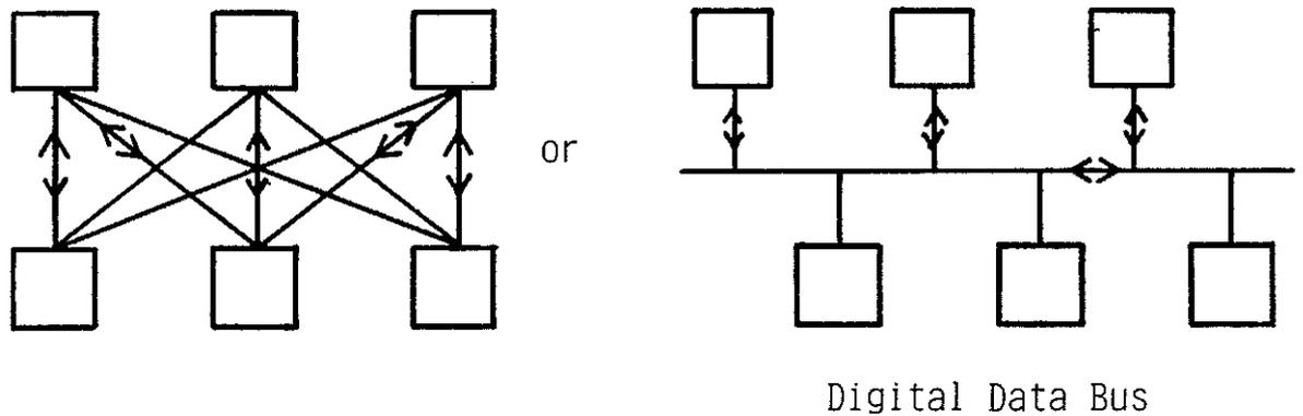
Figure 1. Aircraft Data Transmission Architectures
