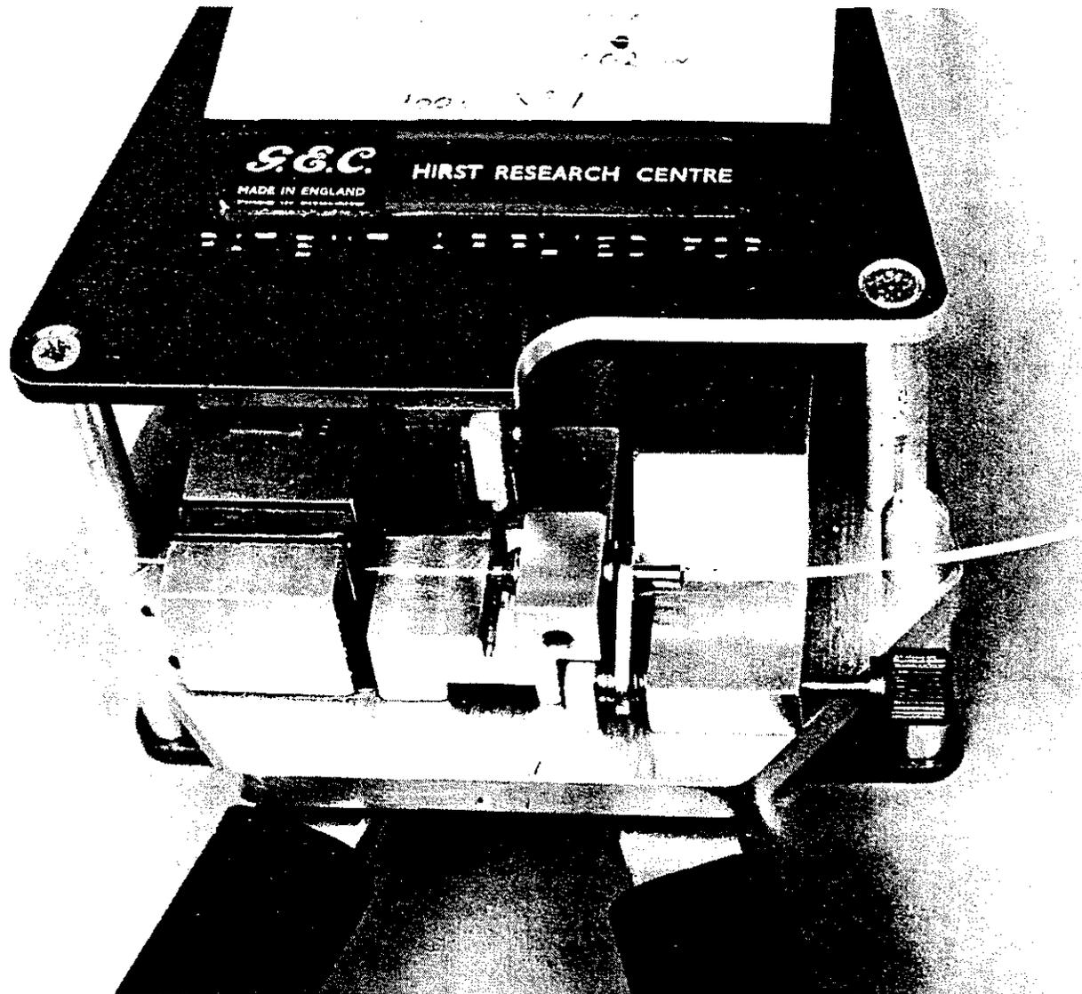
Figure 9. Fibre/Ferrule Assembly in Cleaving Tool Prior to Cleave
