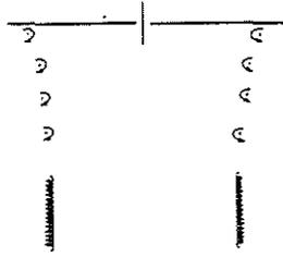
FIG. 2: GEOMETRY OF MODEL USING LINE VORTICES AND VORTEX SHEETS TO REPRESENT THE WAKE.
