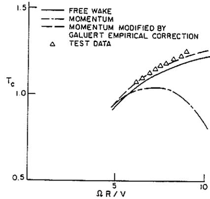
FIG. 8: WIND TURBINE PERFORMANCE PREDICTIONS IN TURBULENT WAKE/VORTEX RING STATE AND COMPARISON WITH EXPERIMENTAL RESULTS OF REF. 15.
