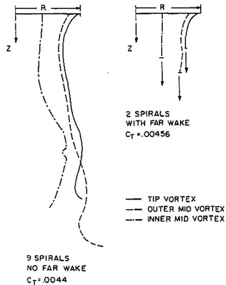
FIG. 5: EXTENDED INTERMEDIATE WAKE FOR TWO BLADED ROTOR OF FIG. 4.
