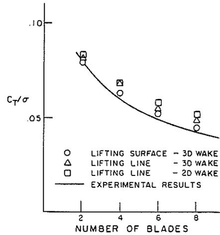
FIG. 7: EFFECT OF BLADE AND WAKE MODELING WITH INCREASING NUMBER OF BLADES AND COMPARISON WITH EXPERIMENTAL RESULTS OF REF. 2, FIG. 16b,  $\theta_{75} = 8^\circ$ .
