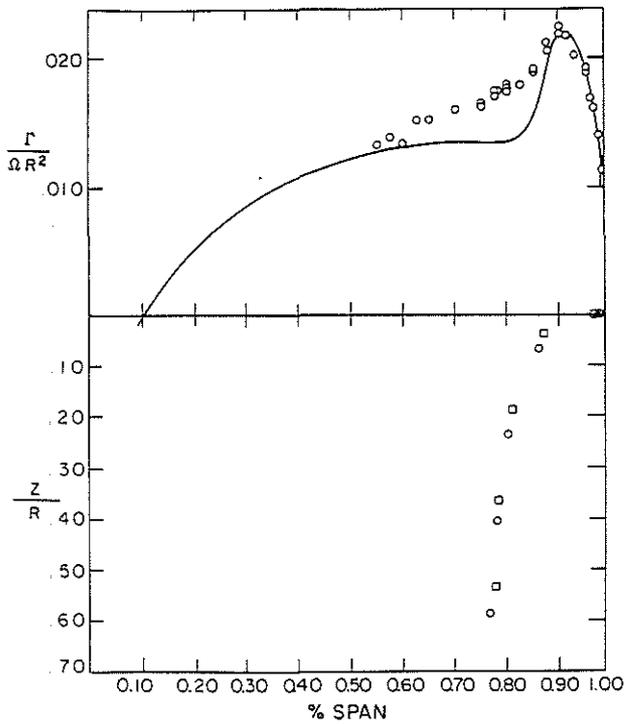
FIG. 6: BLADE BOUND CIRCULATION DISTRIBUTION AND LOCATION OF VORTICES IN WAKE FOR ROTOR OF FIG. 4, BUT WITH EFFECT OF FOLLOWING BLADE TRAILED VORTEX NEGLECTED.
