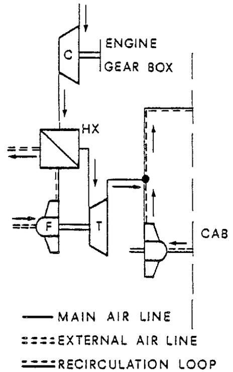
Fig. 6 - Recirculating Shaft Driven Turbofan (RSTF)
