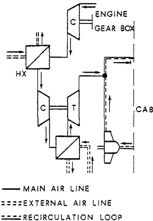
Fig. 7 - Recirculating Shaft-Driven Boot-strap (RSBS)
