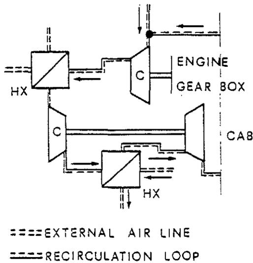
Fig. 11 - Compressed Recirculated Boot-strap (CRBS)
