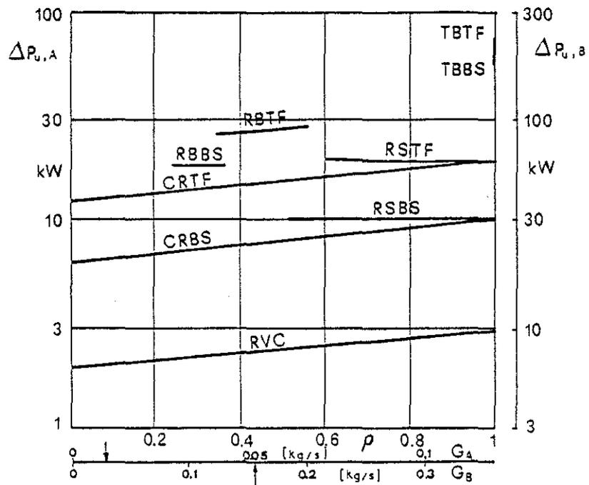
Fig. 14 - Power Consumption for two typical Helicopter ECS
