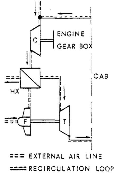
Fig. 10 - Compressed Recirculated Turbofan (CRTF)
