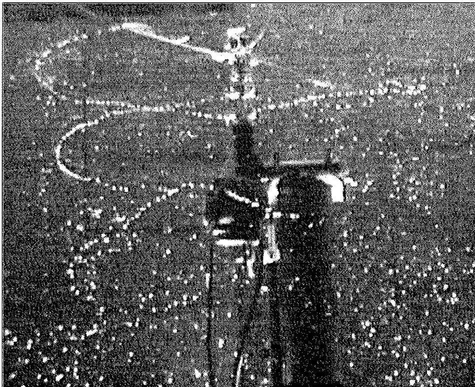
Figure 6 Tip Vortex Structure - Front View
