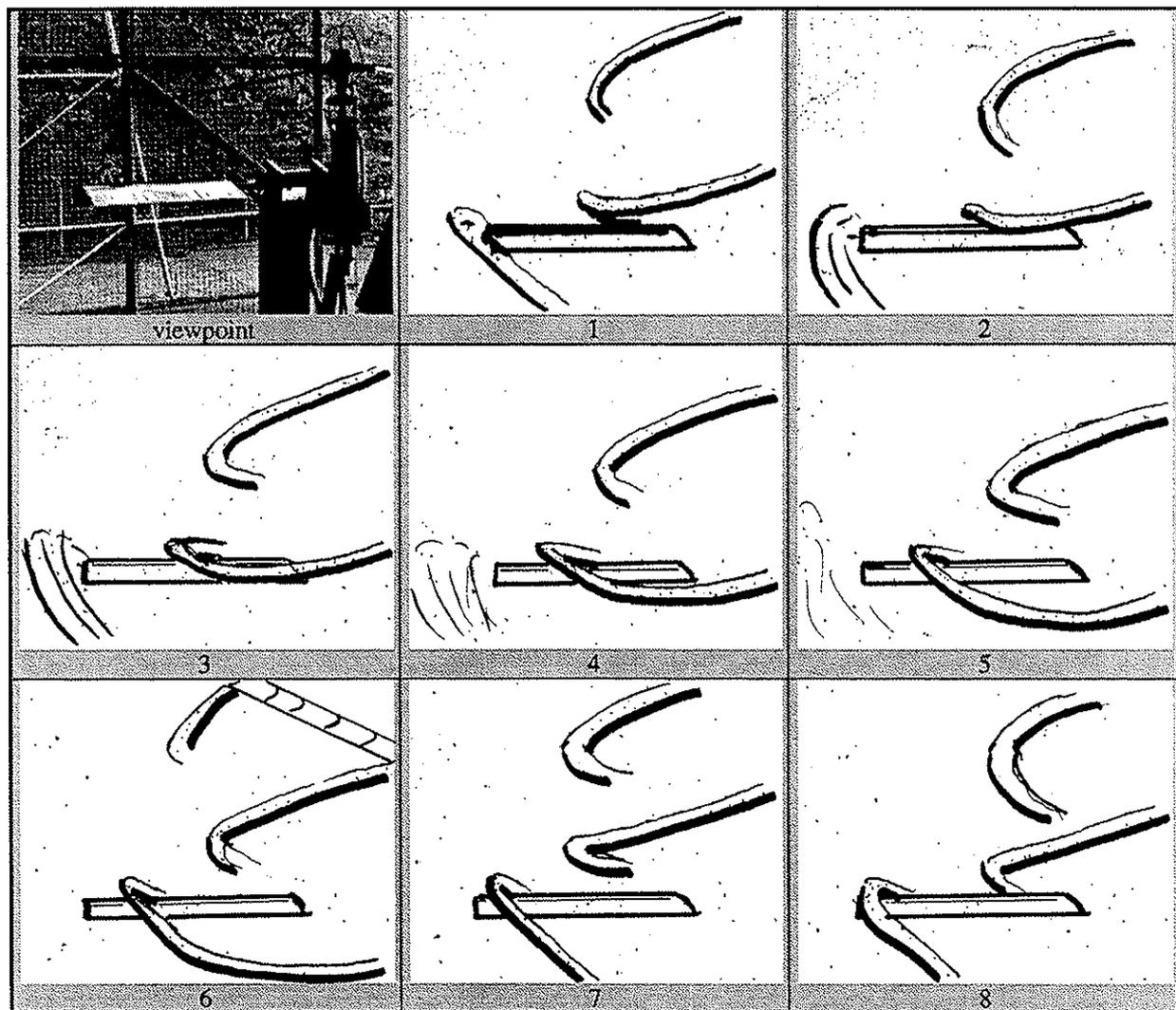
Figure 9 Vortex-Wing-Interaction - Rear View
