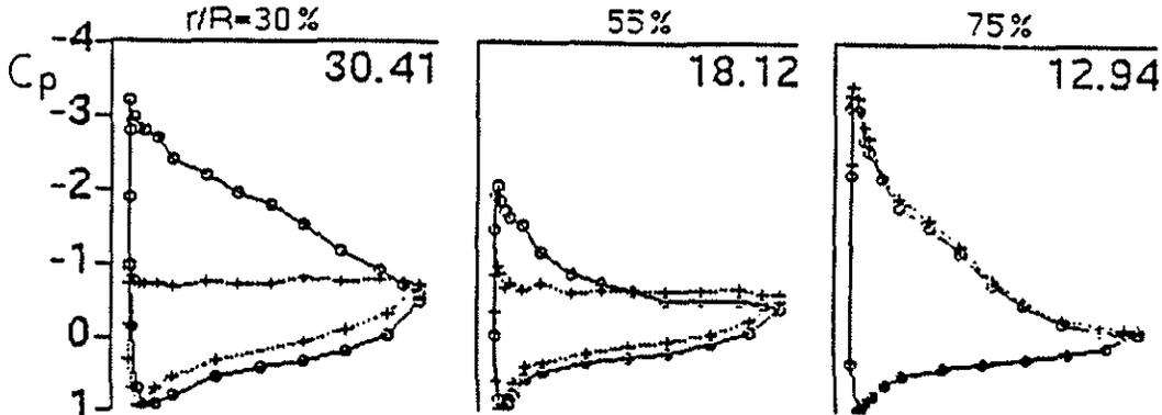
Fig.8: Experimental pressure distributions for the rotating blade (circle) and the non-rotating blade (cross).
