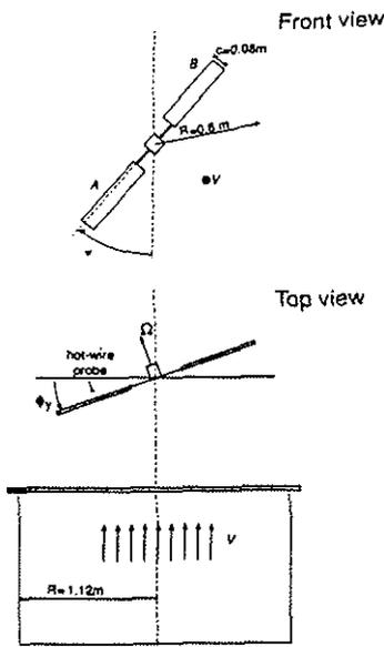
Fig. 5: Windtunnel setup and notations.
