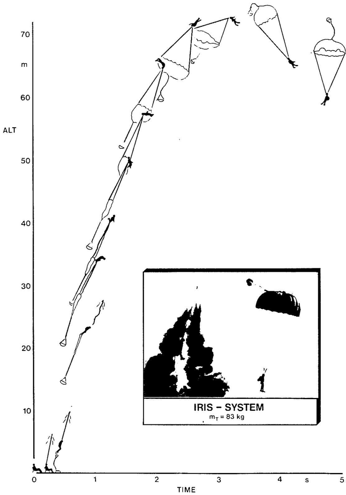
Figure 4. IRIS: Altitude vs. Time during o/o-Test
