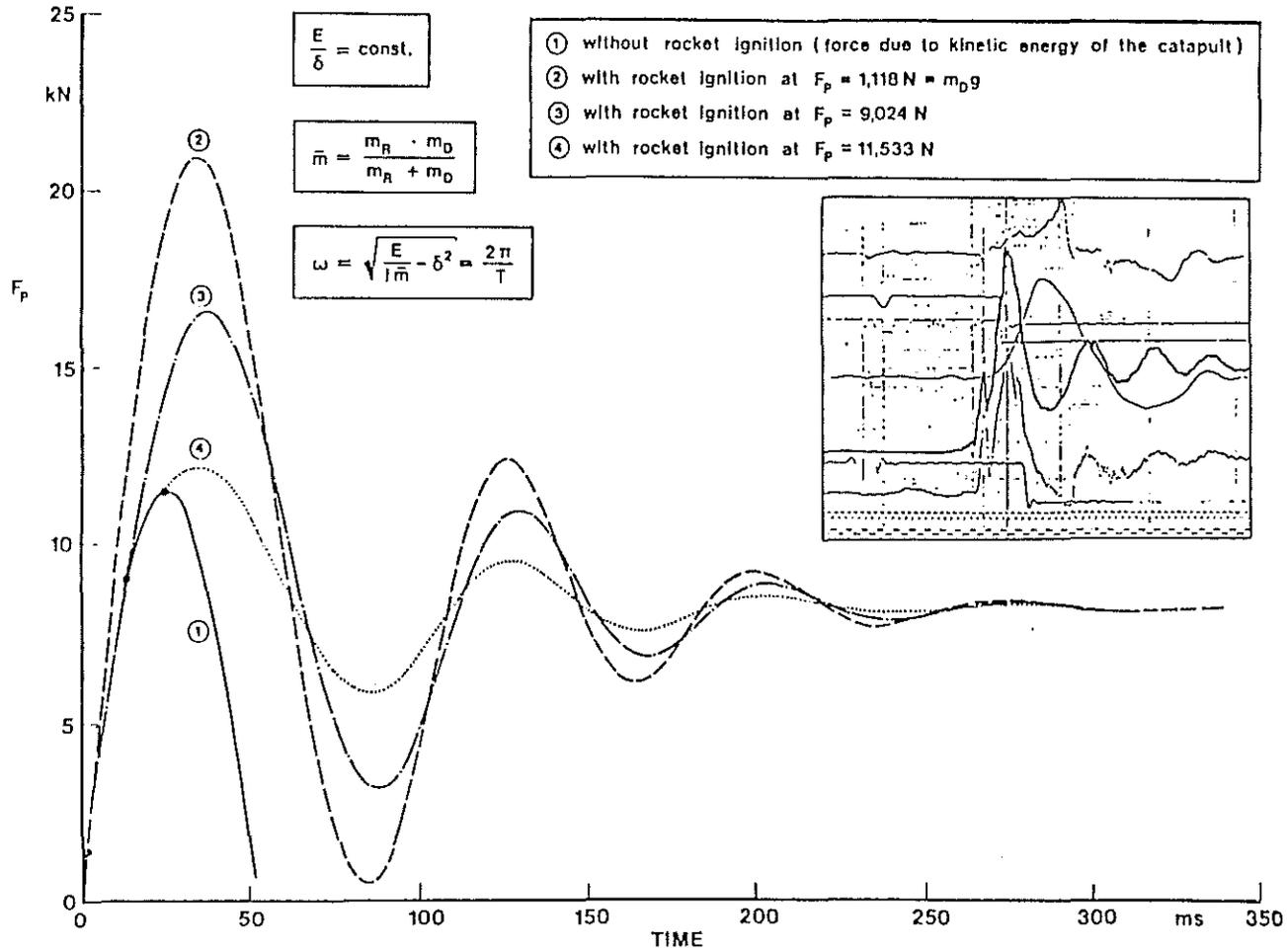
Figure 5. Force vs. Time for Pendant Line
