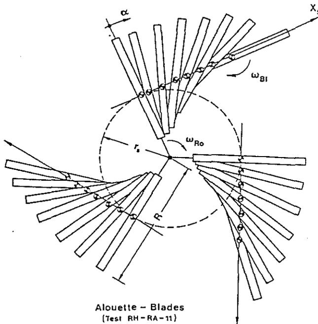
Figure 2. Rotor Blade Removal from Tethered Helicopter
