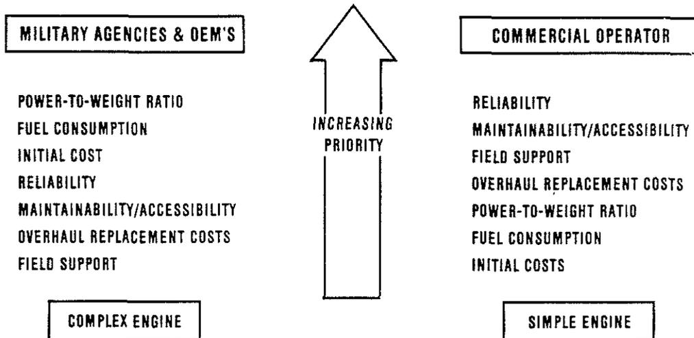
Figure 2. Advanced Helicopter Engines--Market Drivers-Engine Parameters.
