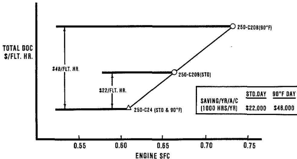
Figure 8. Light Twin Helicopter--Comparative Fuel Costs.
