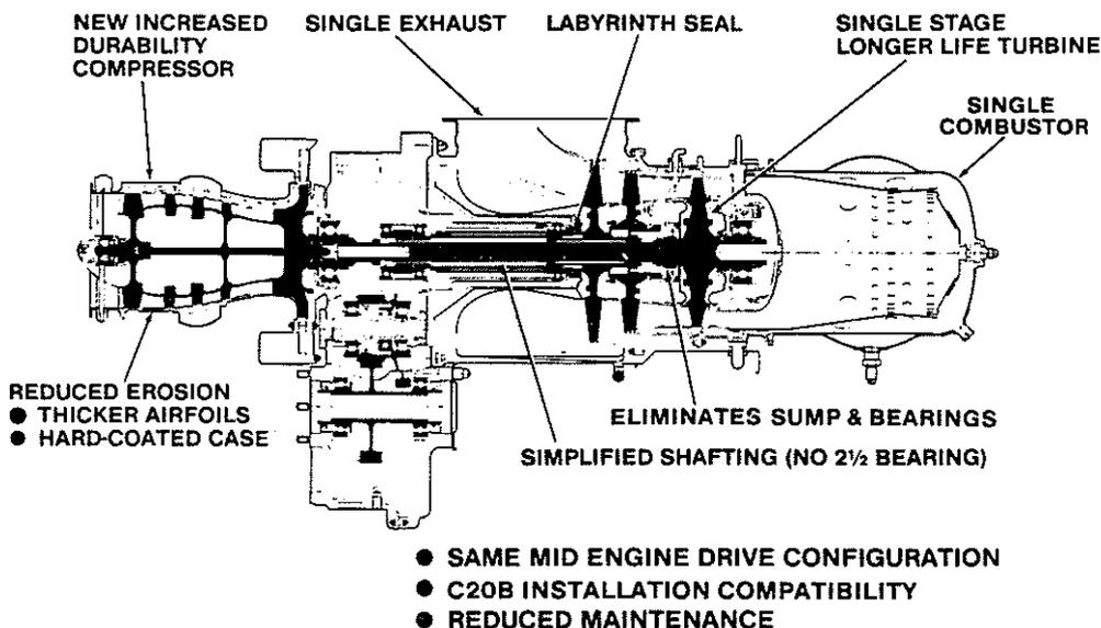
Figure 9. Model 250-C24 Cross Section.
