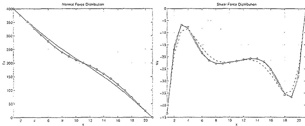
Figure 5: Adherend  $T_x$  and  $V_x$  for different laminates layout with adherends thickness of 1 mm
