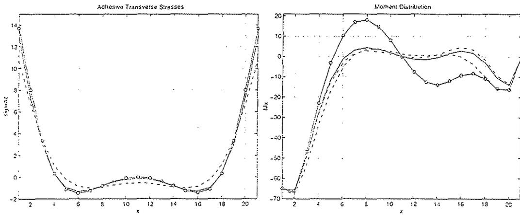
Figure 4: Adhesive  $\sigma_y$  in transverse direction and moment  $M_x$  distribution with adherends thickness of 1 mm
