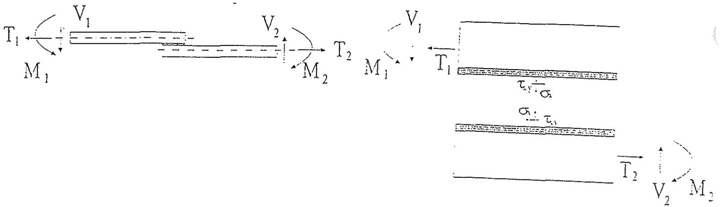
Figure 1: Geometry of the joint and loading conditions
