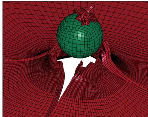
Figure 6. Simulation of the impact of a blunt body against a thin plate.
