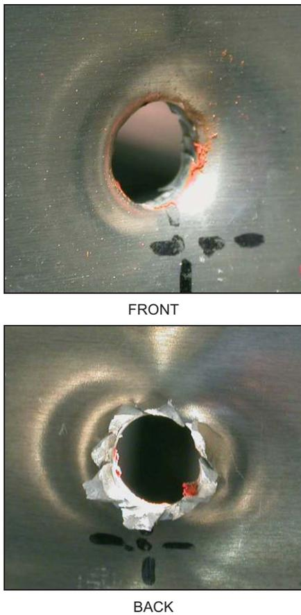
Figure 5. Views of the thin target plate after the impact.
