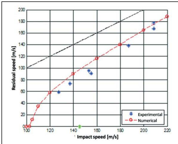
**Figure 12. Impact speed vs. residual speed for impacts on thin plates.**
