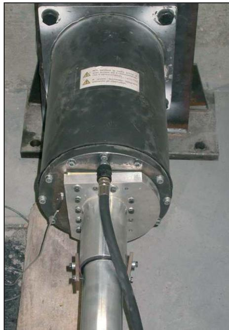
Figure 1. The projectile launcher used in the bullet impact tests.
