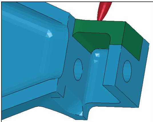
**Figure 14. FE models of the helicopter component and projectile.**
