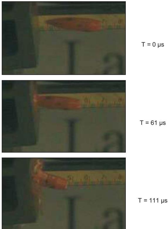
**Figure 16. Impact sequence of test onto the helicopter component.**
