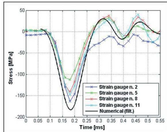
Figure 11: comparison between calculated and measured stresses.
