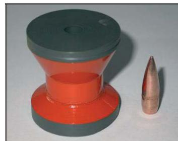
Figure 2. The sabot used in the bullet impact tests and a bullet.
