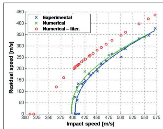
Figure 8. Residual velocity of a blunt body after the impact onto a thick plate.
