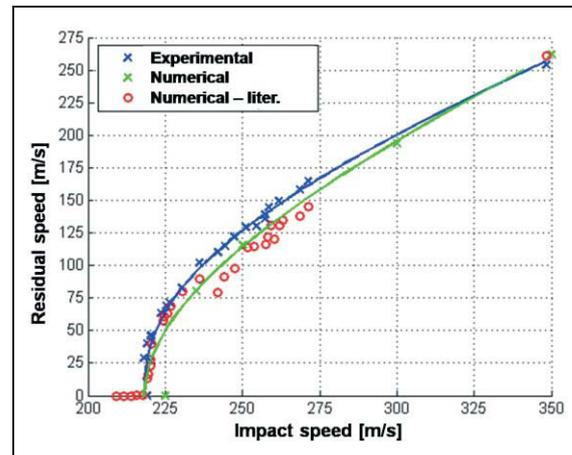
Figure 7. Residual velocity of a blunt body after the impact onto a thin plate.
