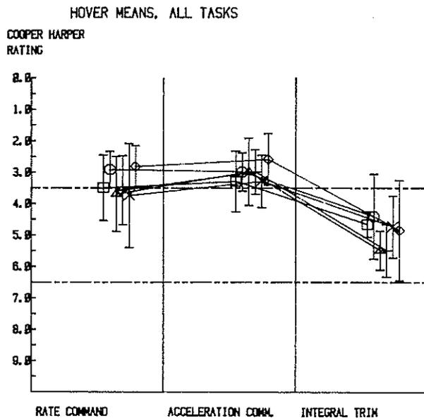
Figure 12: Hover Manoeuvring, Consolidated Data
