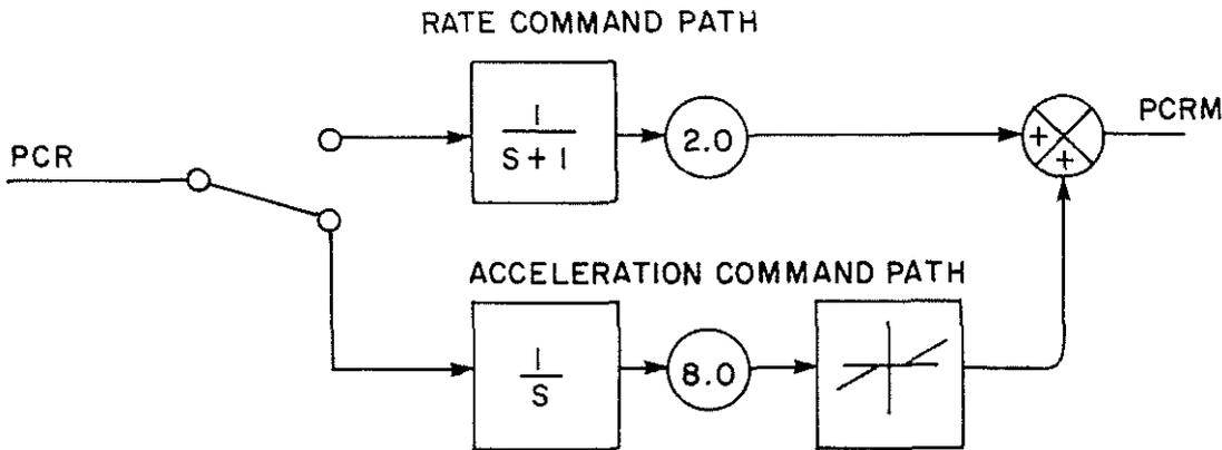
Figure 6: Rate or Acceleration Command Processing
