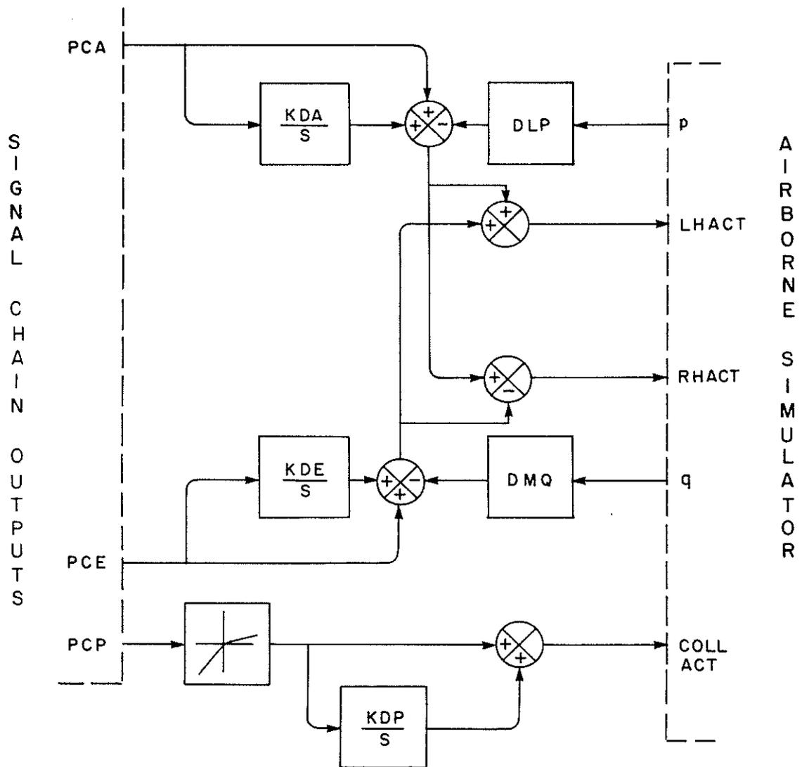
Figure 5: Pitch, Roll and Heave Control Systems
