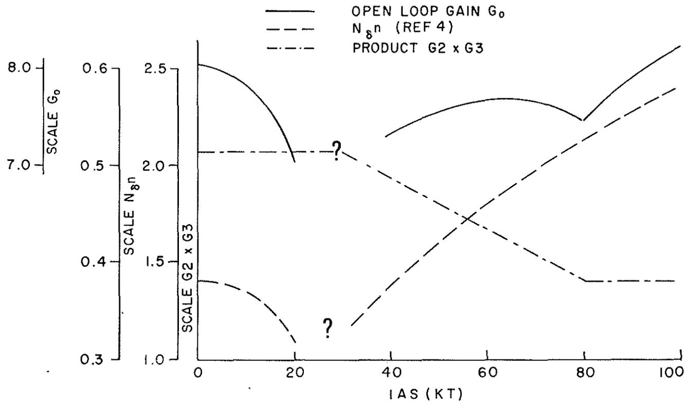
Figure B-1 Yaw Control System, Open-Loop Gain
