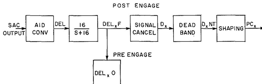
Figure 3: The Signal Pre-Processing Chain
