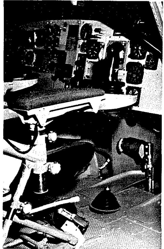
Figure 2: The Controller Mounted in the Airborne Simulator
