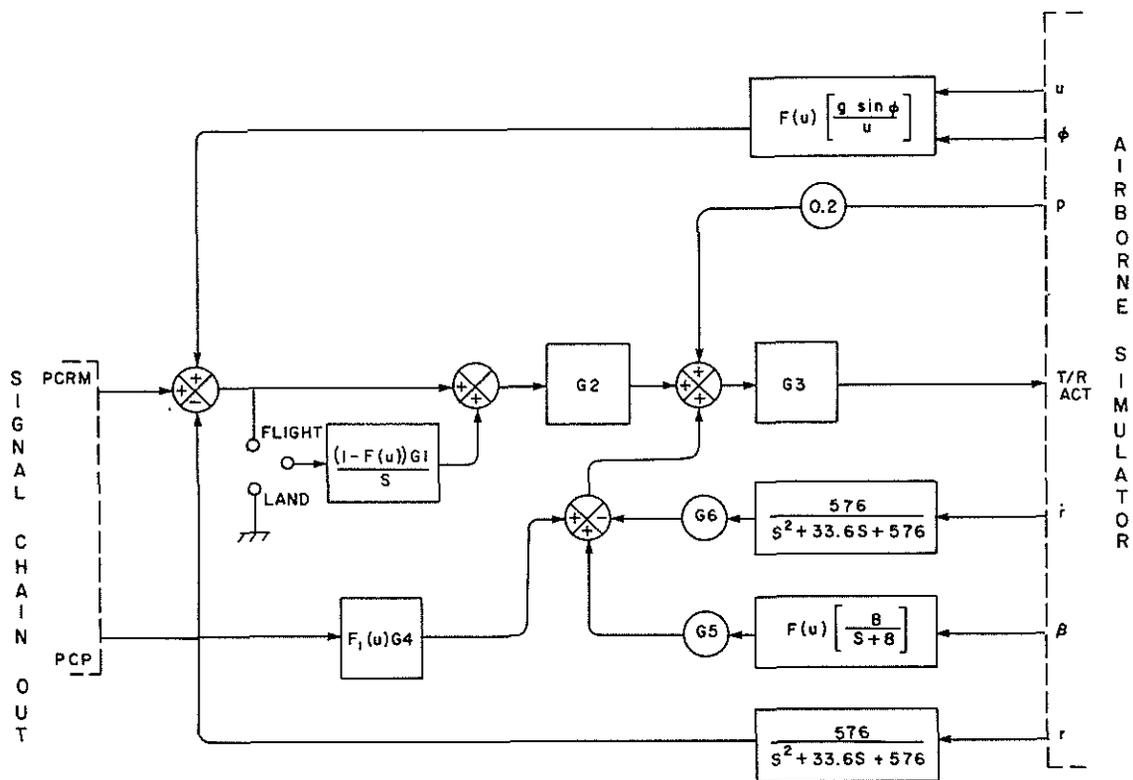
Figure 7: The Yaw Rate-Following Control System
