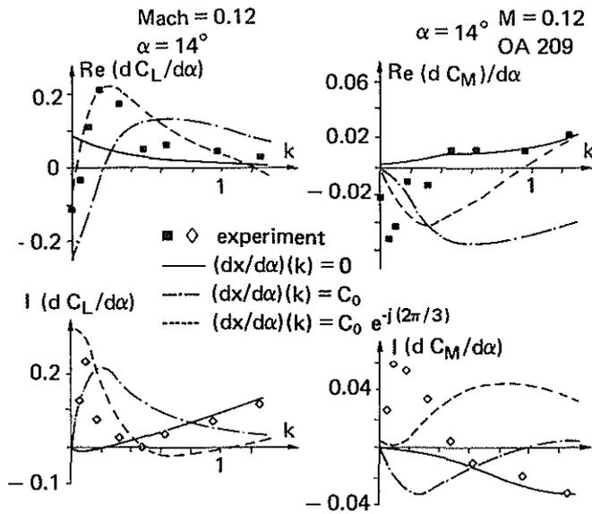
Fig. 13 — Real and imaginary parts of  $dC_z/d\alpha$  and  $dC_M/d\alpha$ . Mean incidence  $14^\circ$ ; oscillations  $\pm 1^\circ$ ;  $k = \omega c/2U_\infty$  (reduced frequency). OA 209 profile Mach = 0.12.
