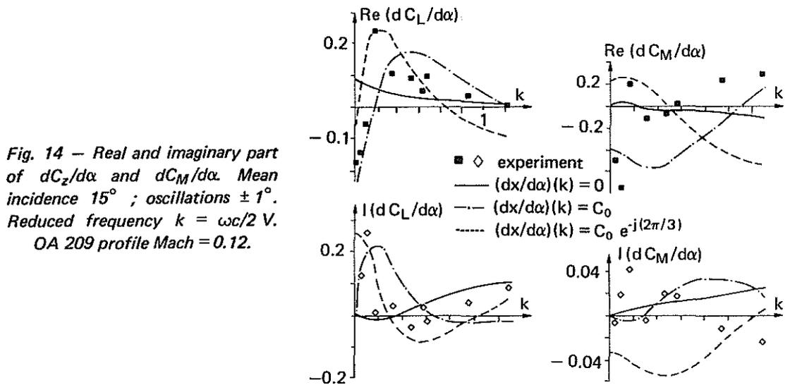
Fig. 14 — Real and imaginary part of  $dC_z/d\alpha$  and  $dC_M/d\alpha$ . Mean incidence  $15^\circ$ ; oscillations  $\pm 1^\circ$ . Reduced frequency  $k = \omega c/2V_\infty$ . OA 209 profile Mach = 0.12.
