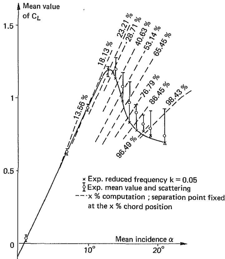
Fig. 12 - Mean value of the lift coefficient when the OA 209 profile is oscillating with an amplitude of  $\pm 1^\circ$  at various frequencies. Mach number 0.12, chord=40 cm.
