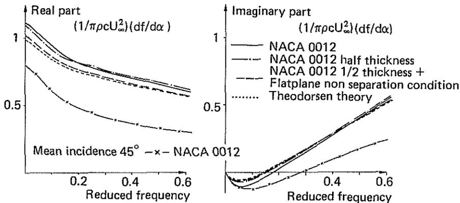
Fig. 5 - Real and imaginary parts of the lift coefficient on various profiles performing small pitch oscillations around a mean incidence of  $0^\circ$  and  $45^\circ$ .
