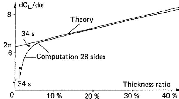
Fig. 3 - The profile is approximated by a polygon with 28 sides and the computed value of  $dC_L/d\alpha$  is compared with the theory. When the number of sides is increased, the results are improved for low thickness ratios. Two results are presented with 34 sides.
