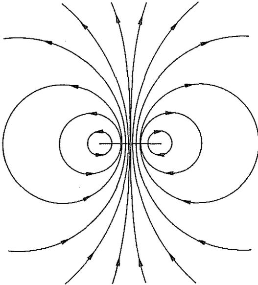
Fig. 1 - Streamlines induced by a segment supporting doublets of constant intensity by unit length.
