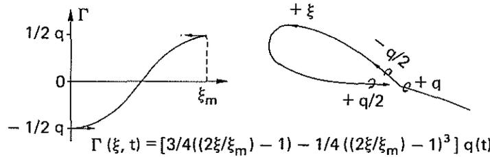
Fig. 4 - Doublets with intensity  $\Gamma(\xi, t)$  are placed on the profile perimeter to counter-balance the wake effect and to introduce a circulation around the profile.
