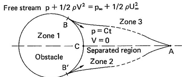
Fig. 6 - Description of a flow around a circular obstacle with separation by means of potential regions.
