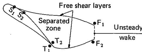
Fig. 11 – Physical scheme used in the case of unsteady computations.
