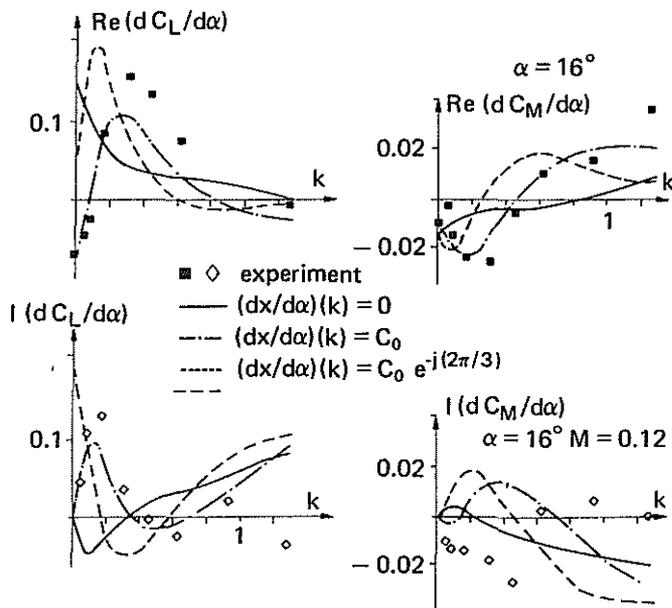
Fig. 15 — Real and imaginary part of  $dC_z/d\alpha$  and  $dC_M/d\alpha$ . Mean incidence  $16^\circ$ ; oscillations  $\pm 1^\circ$ . Reduced frequency  $k = \omega c/2V_\infty$ . OA 209 profile Mach = 0.12.
