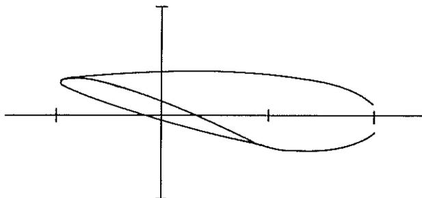
*Fig. 7 – Example of computation for the OA 209 profile. Incidence  $18^\circ$ , separation point 96.49 %, wake length 0.5 chord. Starting from two straight lines, the wake geometry is obtained in 9 steps. Computation time about 4 mn on a CYBER 750.*
