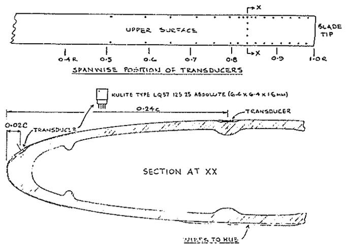
Fig 4 Sensor layout on general research blade
