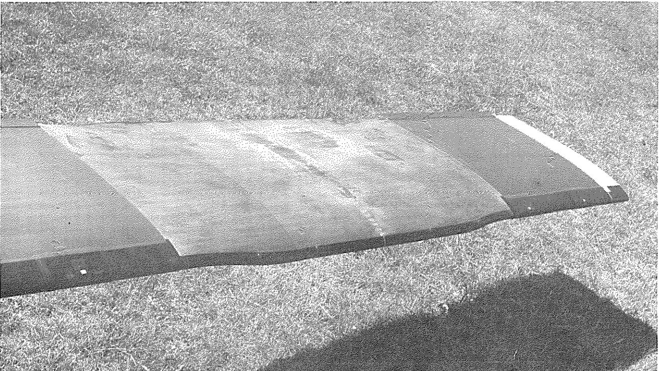
**Fig 6** Experimental aerofoil glove section
