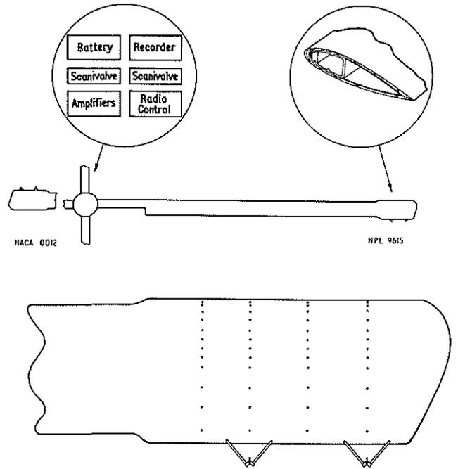
Fig 2 Schematic of aerofoil comparison system
