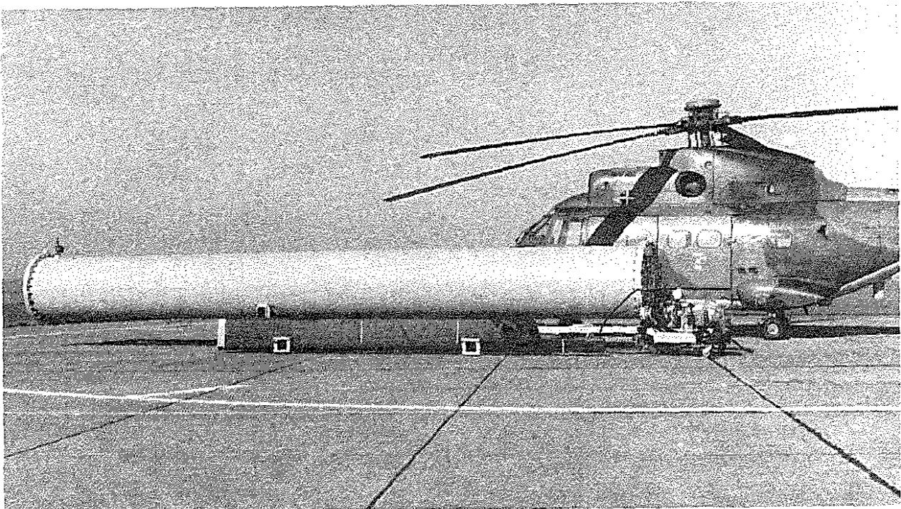
Fig 12 Pressure sensor calibration using the test chamber
