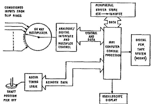
Fig 10 Schematic of digital recording
