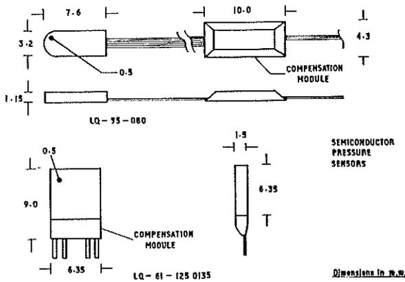
Fig 3 Pressure sensors
