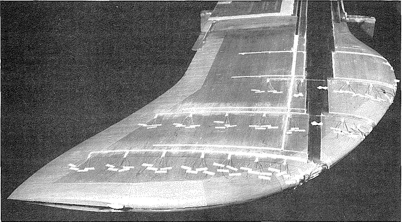
**Fig 5** Swept tip glove under construction
