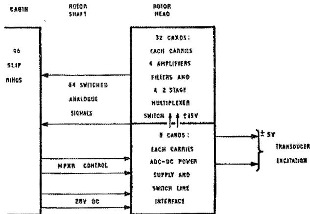
Fig 7 Arrangement of rotor head instrumentation pack
