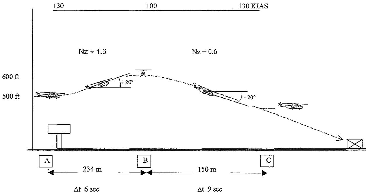
Figure 6: ACHIEVED RESULTS FOR HH-3F Pull up - Push Over flight trials
