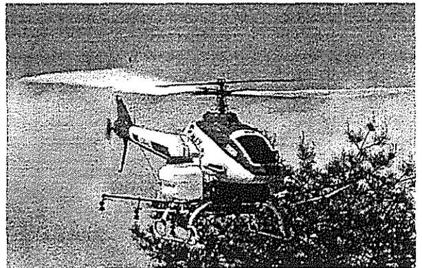
Figure 9. RMAX Remote Controlled Helicopter In Agriculture Spraying Configuration.
