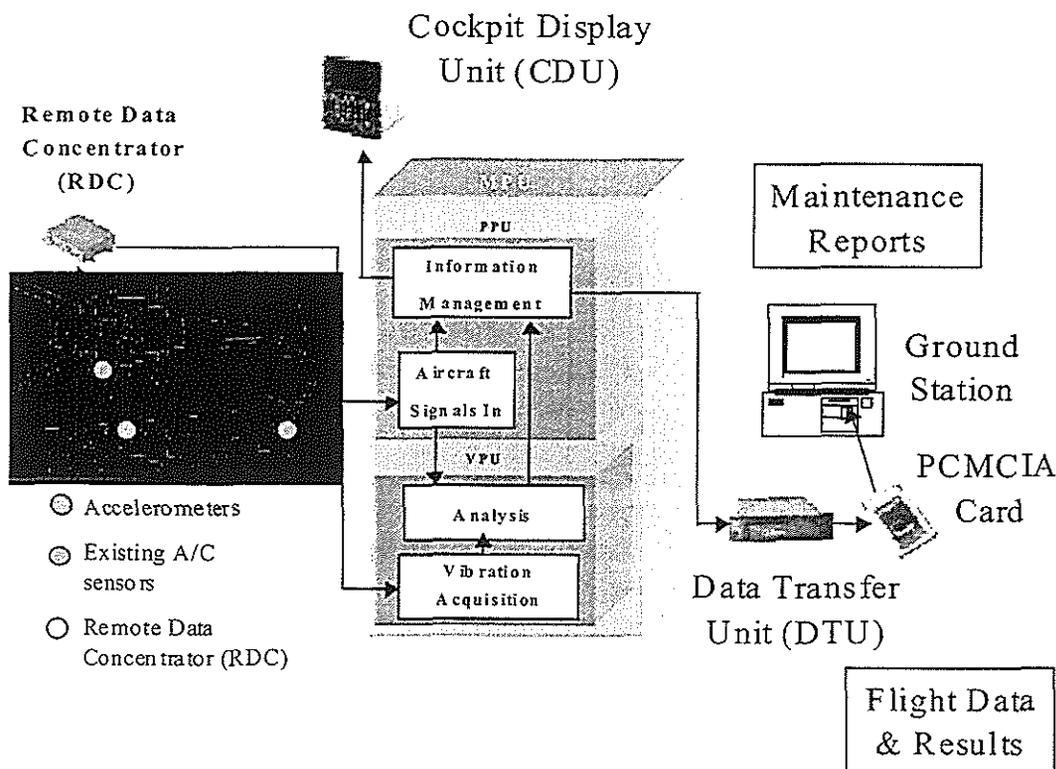
Figure 2. General Configuration of the Airborne System Primary Components
