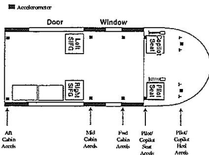
Fig. 7 AVC aircraft installation in a Sikorsky UH-60
