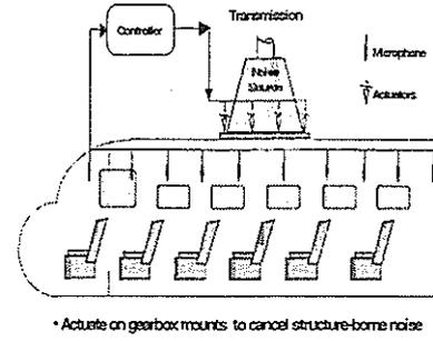
Fig. 2 Control architecture for helicopter gear-mesh ANC
