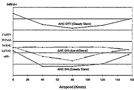
Fig. 11 ANC performance during quasi-steady & transient speed sweep.
