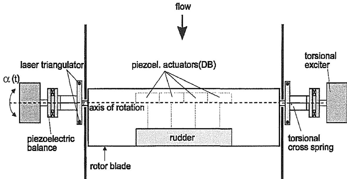
Fig. 5: Test Set-up in the DLR-TWG Wind Tunnel
