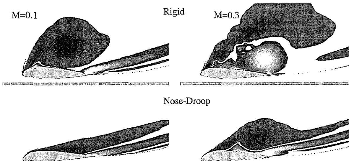
Fig. 2 : Dynamic Stall Control on NACA23012 Airfoil by a Nose-Droop Device
