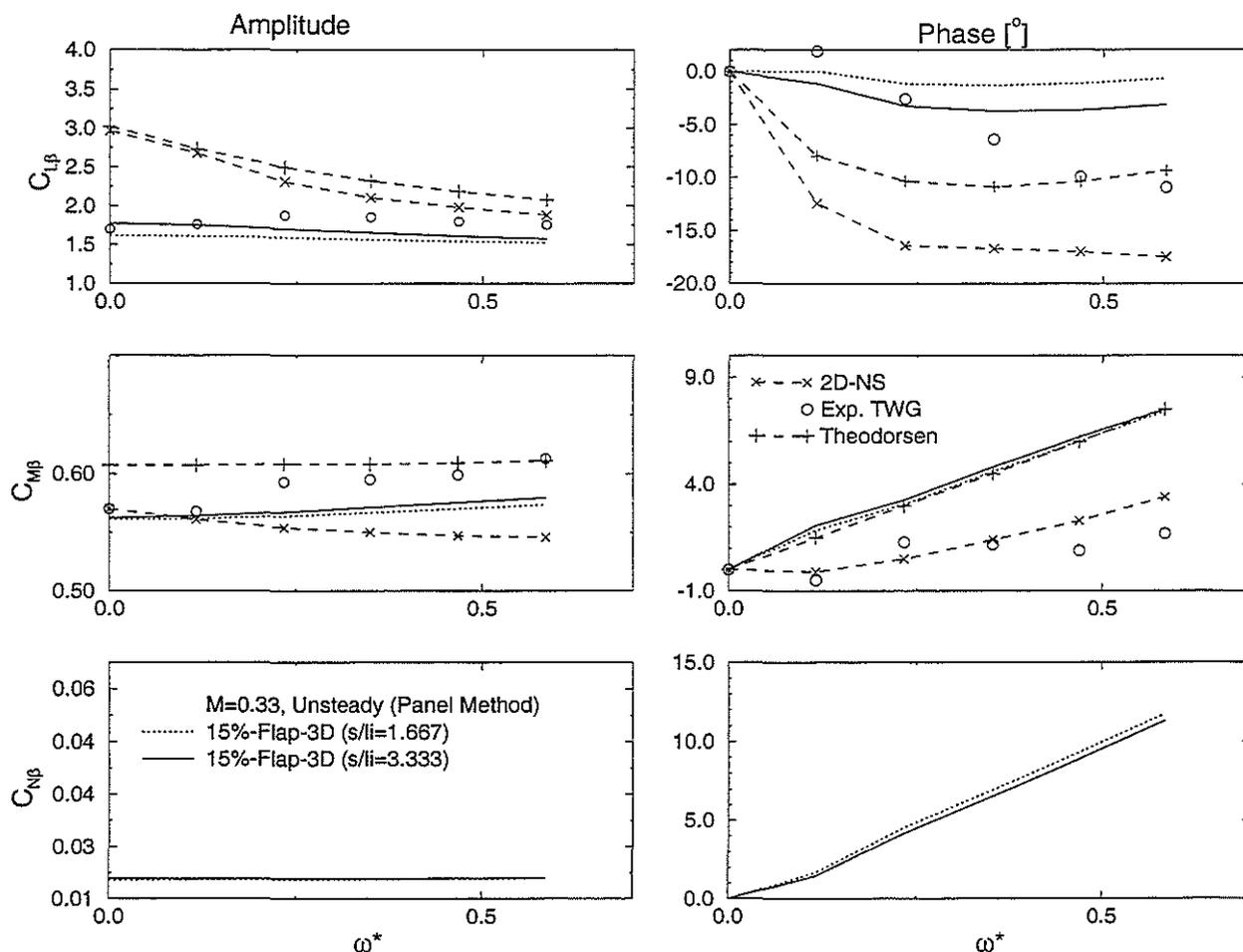
Fig.11: Amplitude and Phase of Flap Efficiency with Respect to Reduced Frequency
