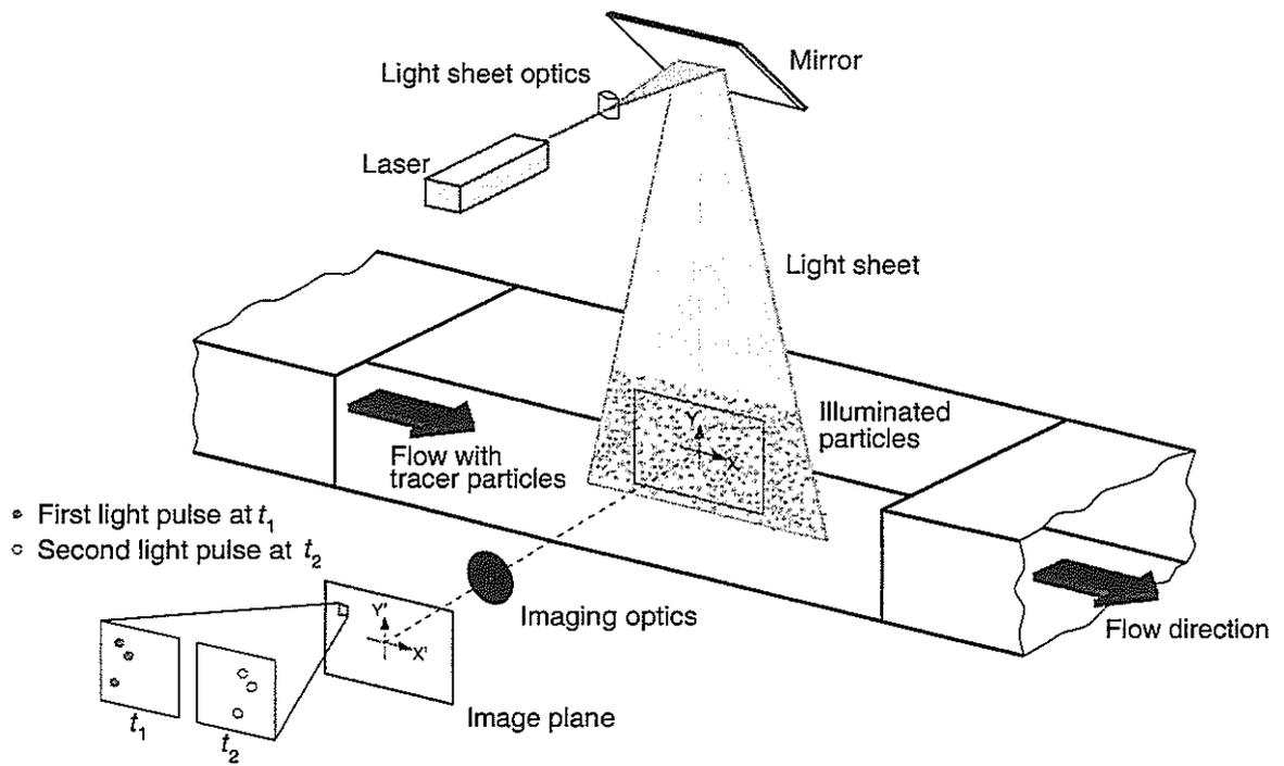
Fig.3: Particle Image Velocimetry for Instantaneous Velocity Field Measurements.
