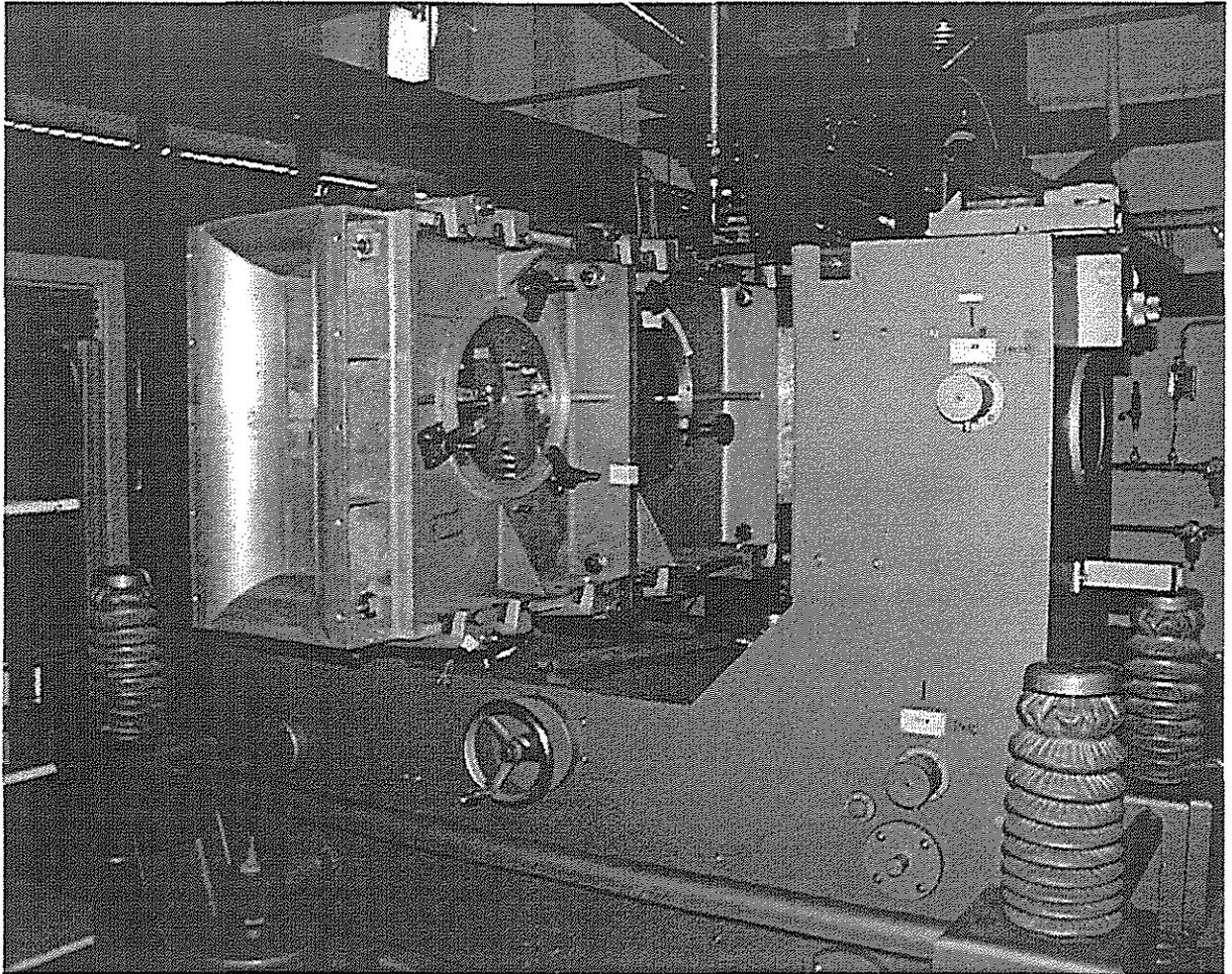
Fig. 8: Research Wind Tunnel VAG equipped with Mach-Zehnder Interferometer and PIV. Investigation of Instantaneous Flow fields at Dynamic Stall and Stall Control
