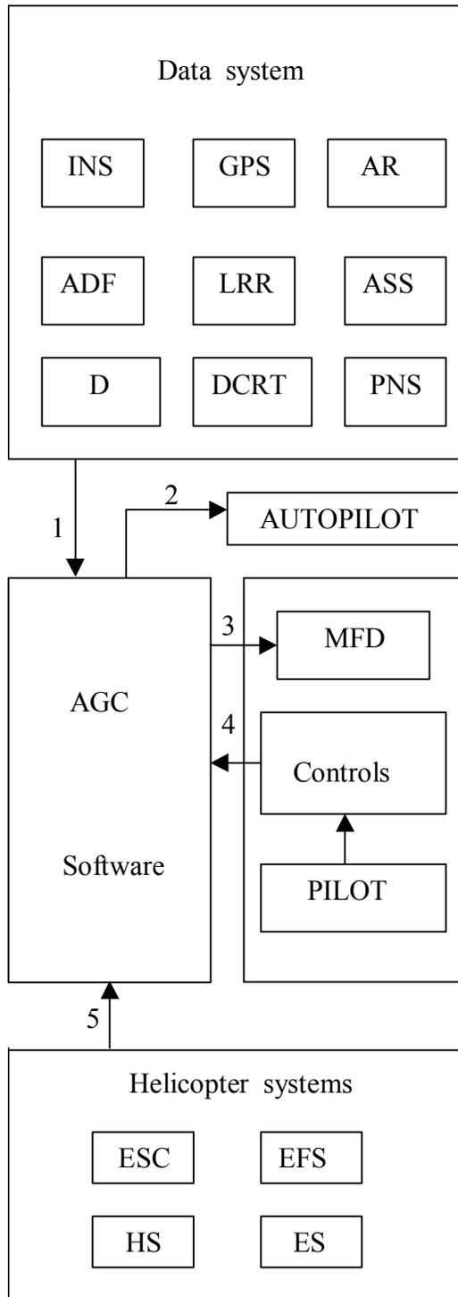
Fig. 1 Frame AEC of the helicopter.
