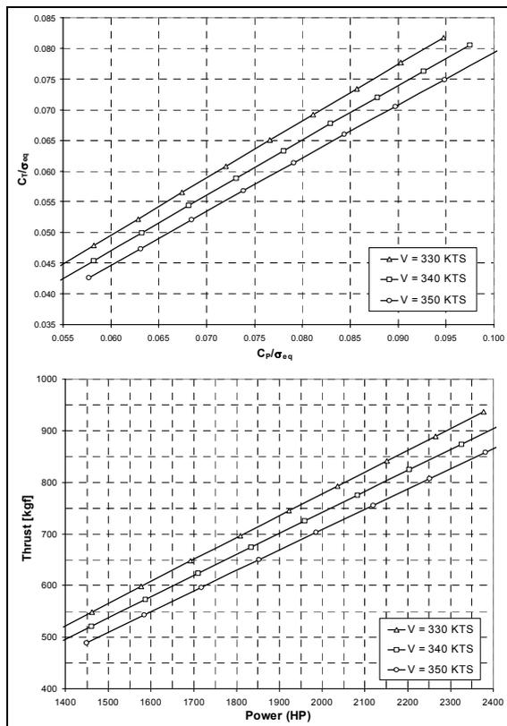
Figure 11: Rotor performance in aircraft mode
