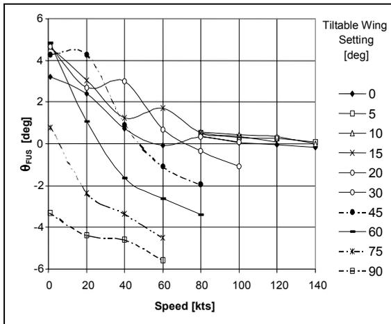
**Figure 28: Aircraft attitude as function of speed and wing tilt angle**
