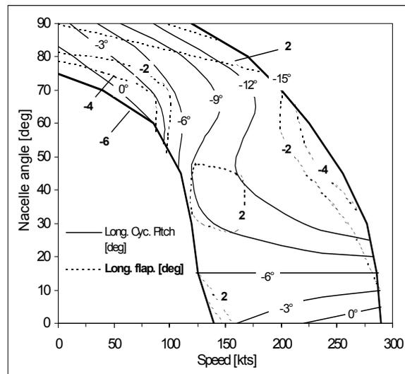
**Figure 30: Conversion corridor vs. long. pitch and flap**
