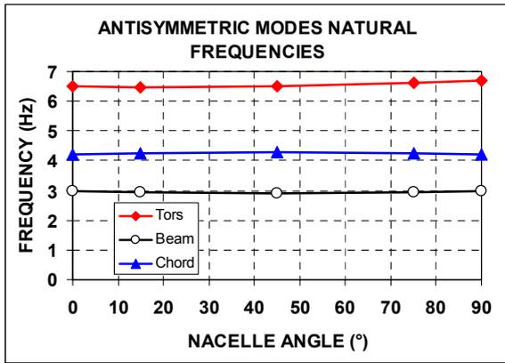
**Figure 18: wing anti-symmetric modes natural frequencies**
