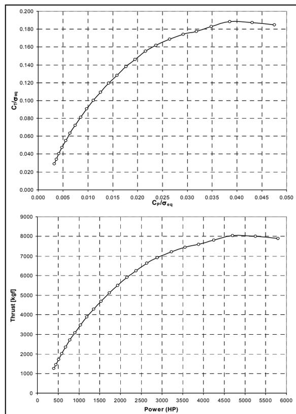
Figure 9: Rotor performance in helicopter mode
