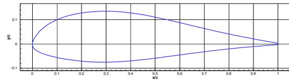
Figure 2: Optimised wing airfoil shape
