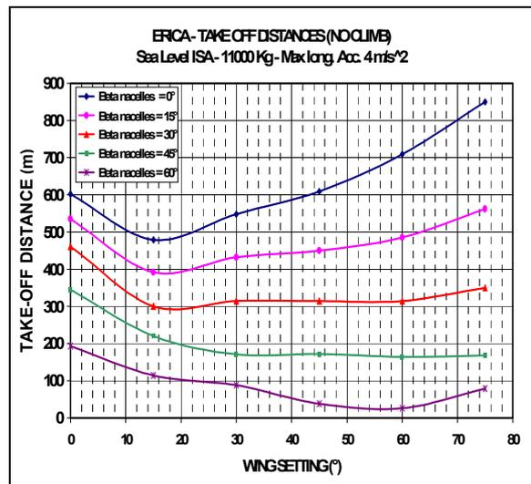
Figure 26: Take off distance vs. tilting wing attitude
