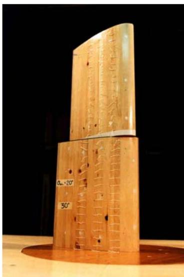
Figure 3: Wind tunnel tests on ERICA wing
