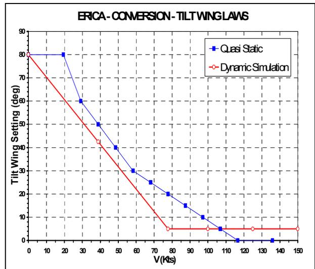
Figure 34: Tilting wing optimised angle
