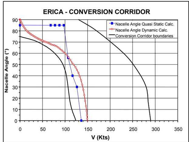
Figure 33: Conversion corridor and optimised path
