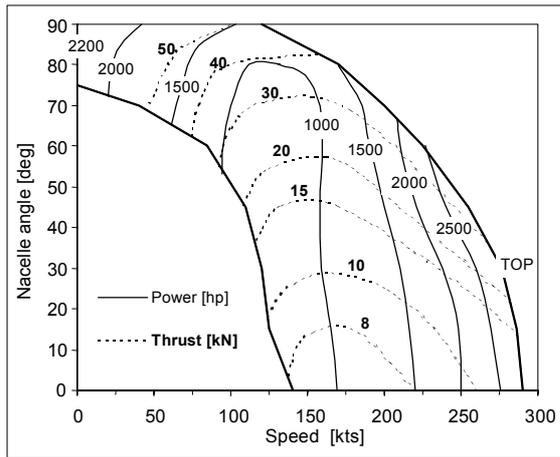
Figure 31: Conversion corridor vs. power and thrust
