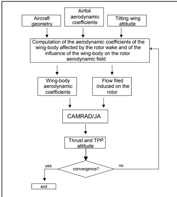
**Figure 27: Process of computation of the performance**
