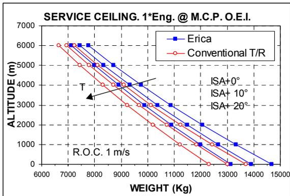
Figure 23: Helicopter mode service ceiling O.E.I.
