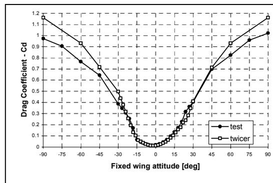
Figure 6: Wing  $C_{d-\alpha}$  for tilt wing at 0 deg.
