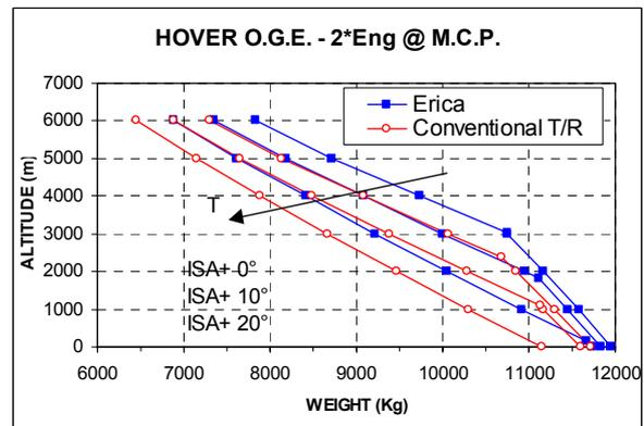
**Figure 20: Helicopter mode HOGE at M.C.P.**
