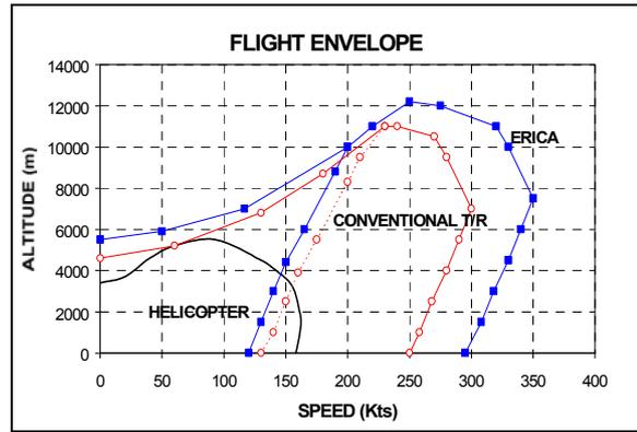
Figure 25: Comparison of flight envelopes
