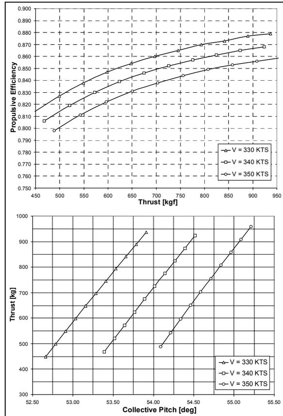
Figure 12: Rotor performance in aircraft mode
