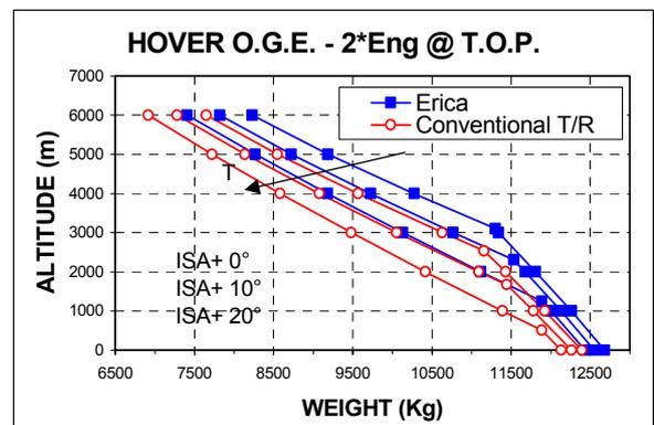
**Figure 21: Helicopter mode HOGE at T.O.P.**
