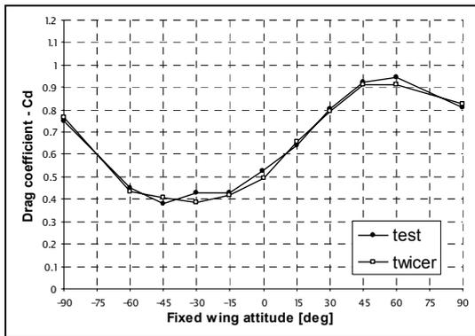
Figure 8: Wing Cd- $\alpha$  for tilt wing at 60 deg.
