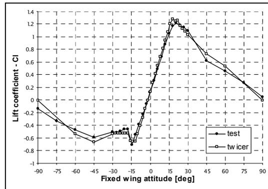
Figure 5: Wing  $C_{l-\alpha}$  for tilt wing at 0 deg.
