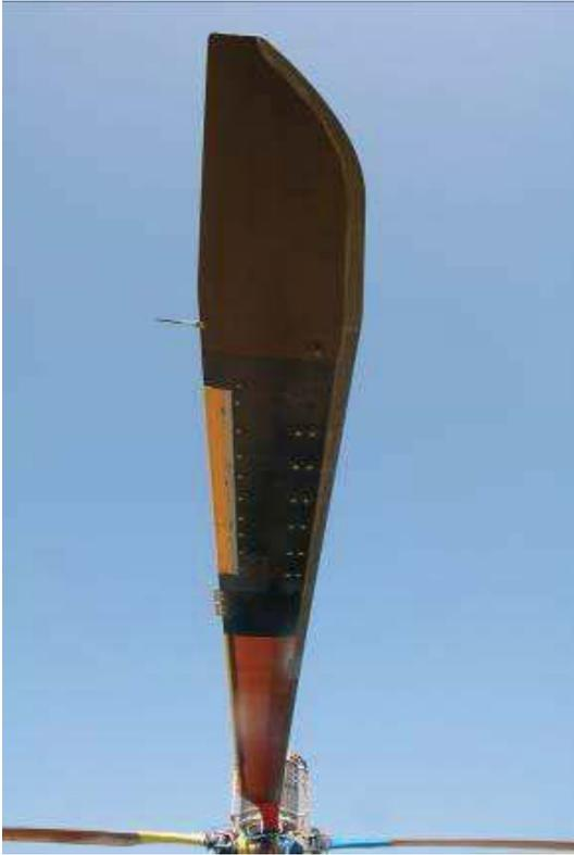
**Fig. 2:** ADASYS rotor blade featuring active trailing edge flaps
