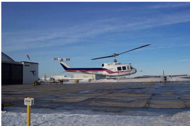
**Figure 1: NRC Bell 205 Airborne Simulator**
