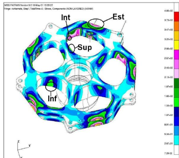
Fig 3: M/R Hub FE Model Stress Analysis
