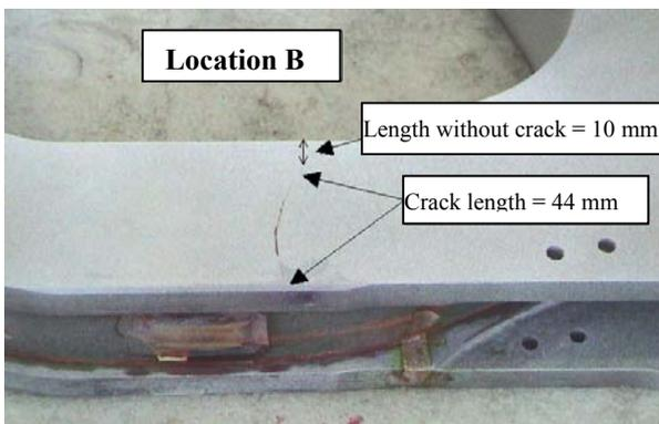
Fig 4: M/R Hub pre-crack for fail safe test
