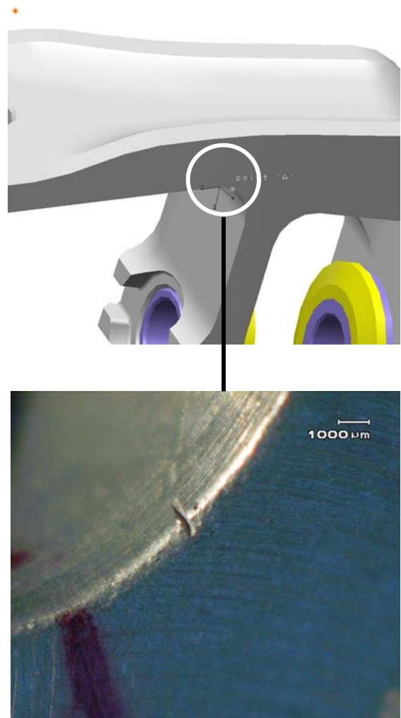
Figure 7: T/R Blade Damper Attachment 0.2 mm initial flaw
