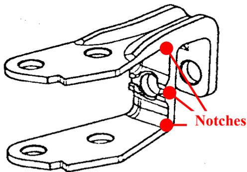
Fig 6: Failures location
