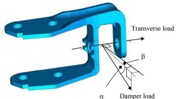
Fig 5: T/R Blade Damper Attachment
