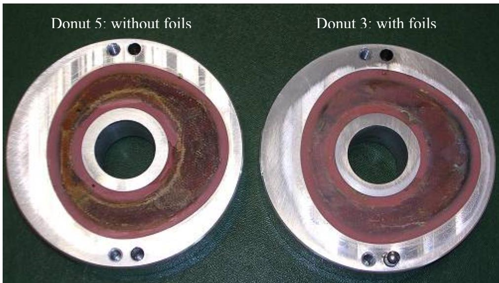
Figure 24: Photo showing the status of the “Donut” specimens with and without separation foils after the dynamic test
