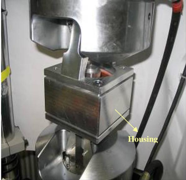
Figure 21: Photo of the test apparatus with specimens already placed into the housing
