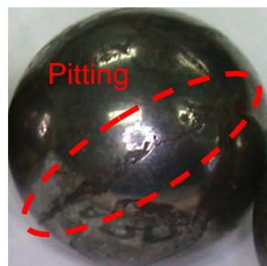
b) Oil Cooler Fan Ball Bearing
