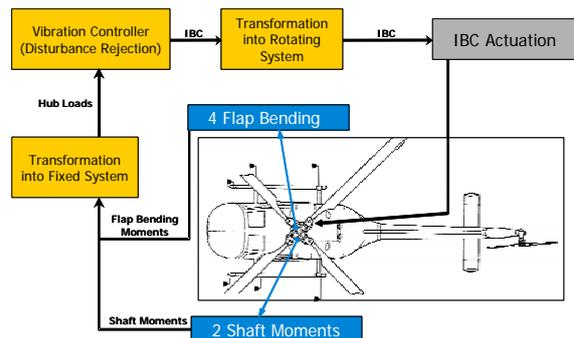
Fig. 14: Schematic view of the vibration control system
