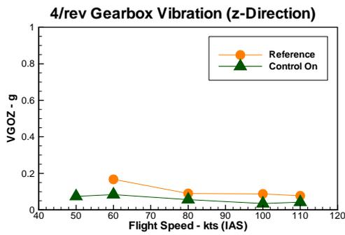
Fig. 22: 4/rev gearbox vibration vs. flight speed (100% rotor speed)
