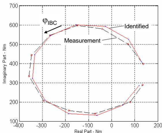
Fig. 19: Comparison of 4/rev pitch moments ( $M_y$ ) at 100 kts (identified vs. measurement)
