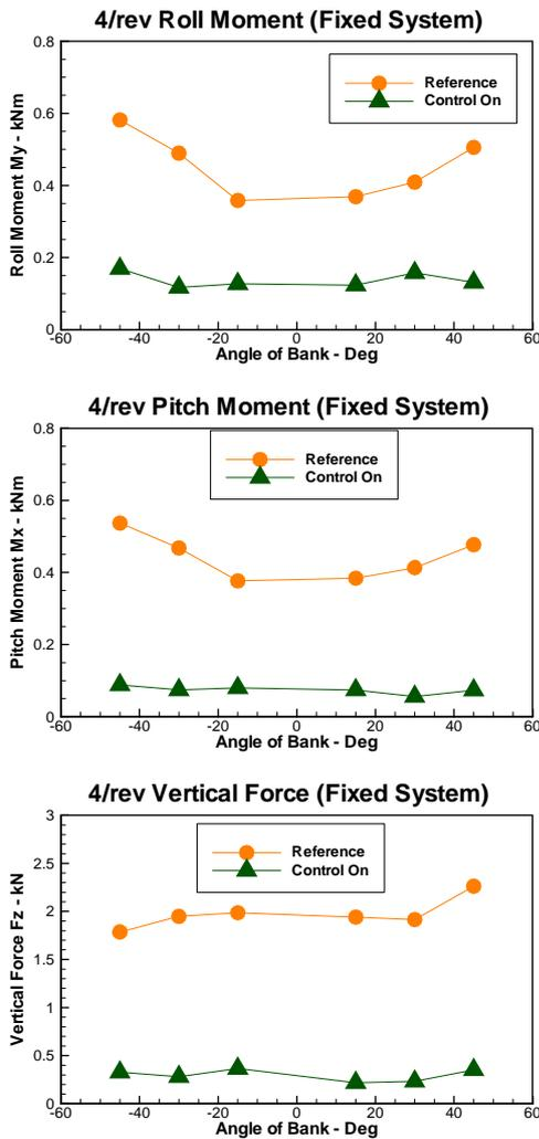
Fig.26: 4/rev hub loads in manoeuvre flight conditions at 80 kts
