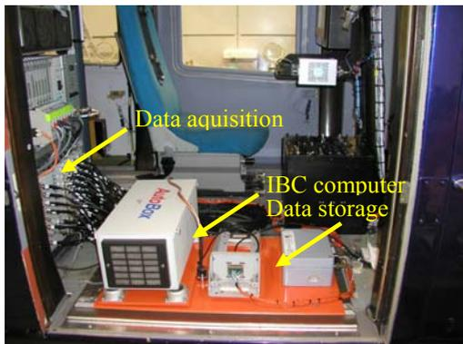
Fig. 9: Integration of the IBC computer and the data acquisition system into the helicopter
