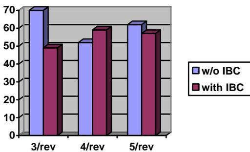
Fig. 27: Lead-lag amplitudes ( $M_c - Nm$ ) with and without IBC at 100kts level flight
