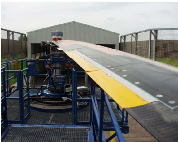
Fig. 7: ECD whirl tower with one pair of ADASYS blades
