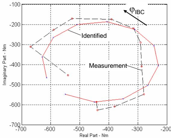
Fig. 18: Comparison of 4/rev roll moments ( $M_x$ ) at 100 kts (identified vs. measurement)
