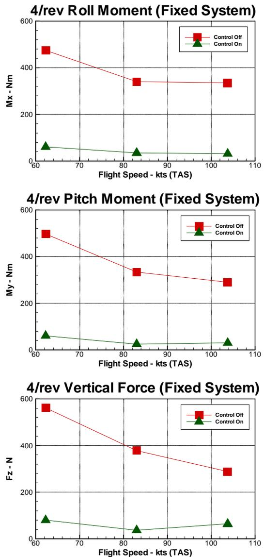
Fig. 3: Controlled hub loads vs. flight speed at nominal rotor speed, BO105 S1
