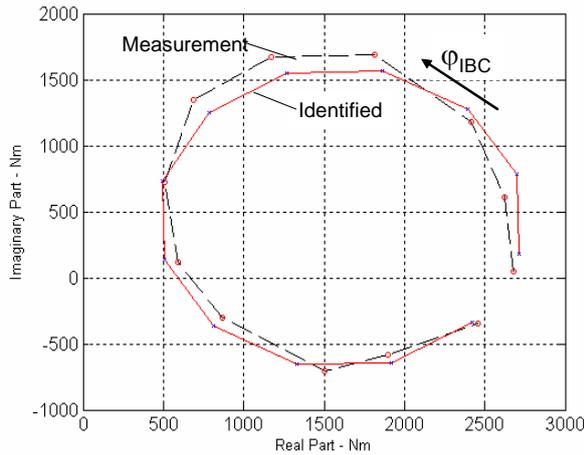
Fig. 17: Comparison of 4/rev vertical forces ( $F_z$ ) at 100 kts (identified vs. measurement)
