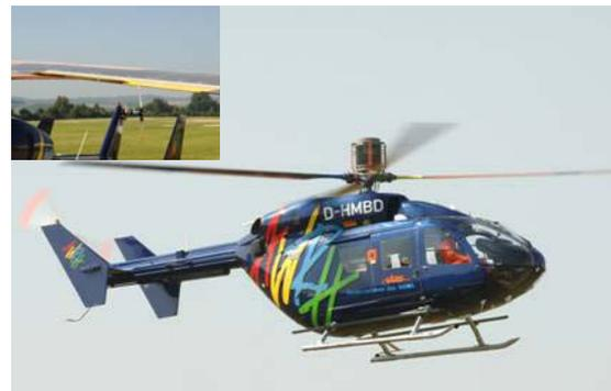
Fig. 11: First flight of a the BK117 S7045 with active trailing edge flaps
