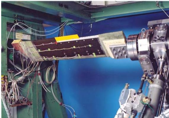
Fig. 6: Blade specimen with active flap during fatigue test
