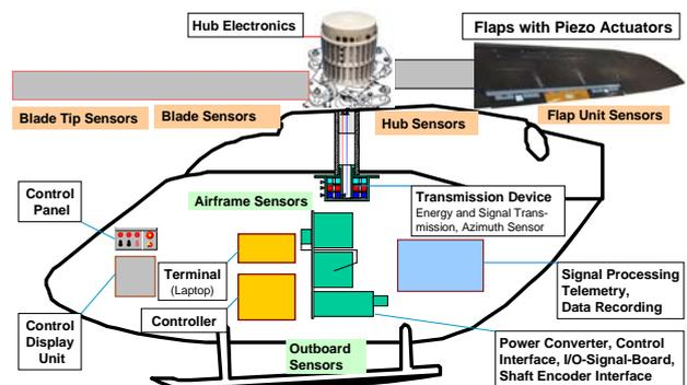
Fig. 8: System architecture of the test helicopter
