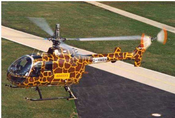
Fig. 1: BO105 S1 IBC demonstrator in flight
