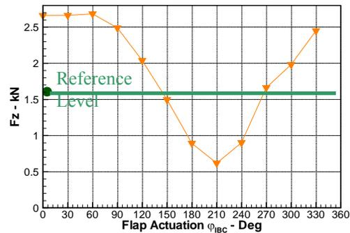
Fig. 16: Vertical hub force in dependence of the IBC phase in level flight (100kts)
