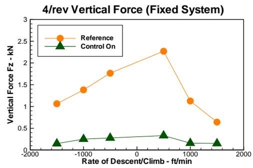
Fig. 24: 4/rev hub loads vs. rate of climb/descent at 65 kts
