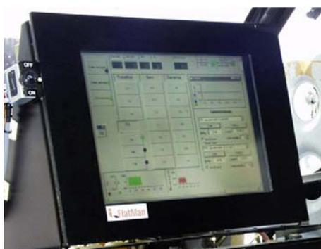
Fig. 10: Touch screen with the control panel
