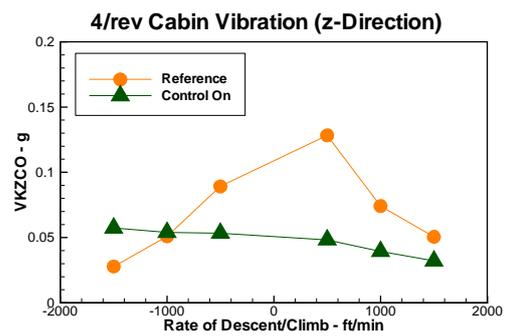
Fig. 25: 4/rev cabin vibration (z-direction) vs. rate of climb/descent at 65 kts
