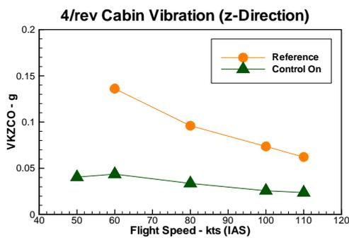
Fig. 23: 4/rev cabin vibration (z-direction) vs. flight speed (100% rotor speed)
