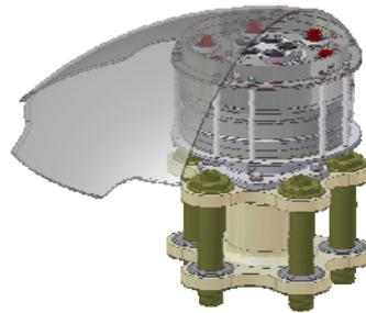
Fig. 28: Hub compartment beneath the hub cap
