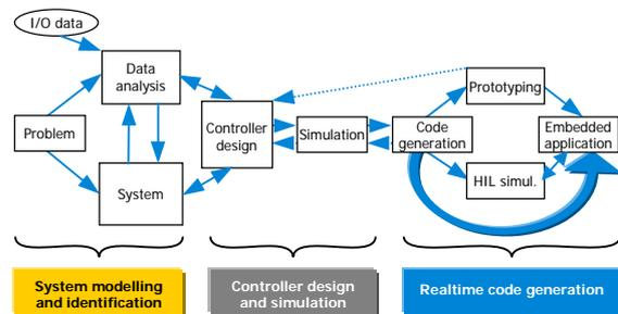
Fig. 13: Realtime controller realisation
