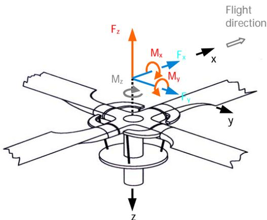
Fig. 2: Hub loads for feedback control
