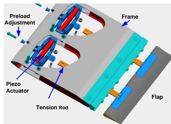
Fig. 5: Flap unit assembly
