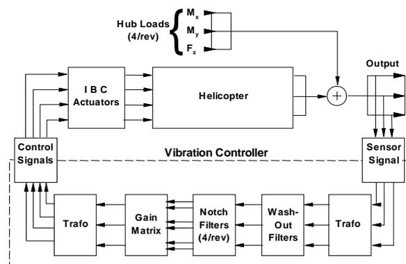
Fig. 12: Feedback loop for 4/rev hub load disturbance rejection (fixed system)
