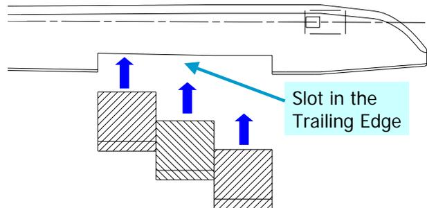
Fig. 4: Installation of the flap units from the trailing edge side
