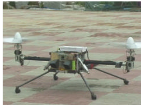
Fig. 12 Frame vehicle in hovering test
