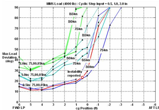
**Figure 6** Effect of varying pilot control inputs on maximum load position deviations
