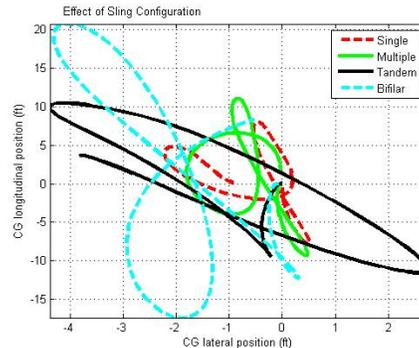
**Figure 10** Effect of rigging configuration on maximum load oscillations
