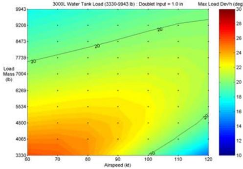
**Figure 3** Maximum load position deviation as a function of airspeed and load mass
