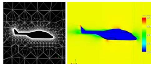
**Figure 15** Mesh domain (left) and velocity field (right) at a representative operational airspeed of 80 knots for the MRH 90
