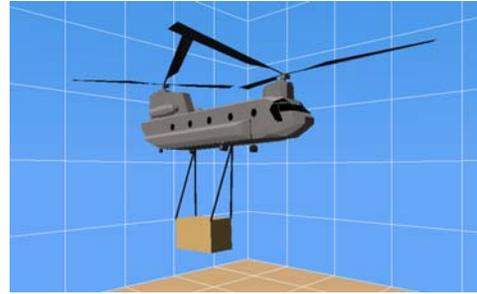
**Figure 4** CH-47D carrying an MMS
