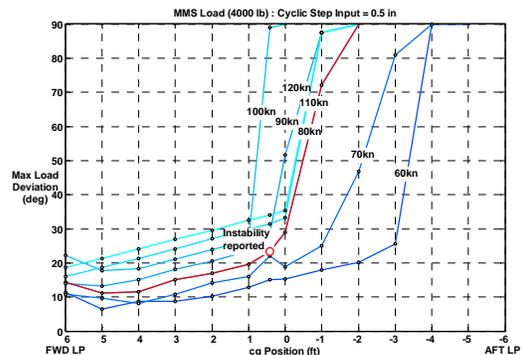
**Figure 5** Effect of varying cg on maximum load position deviations
