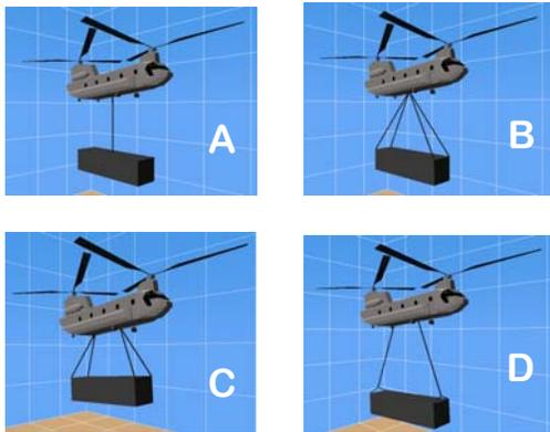
**Figure 9** Rigging configuration; A single point, B multiple point, C tandem and D bifilar
