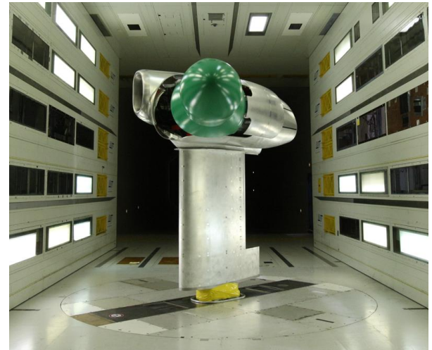
Fig. 8 Full-scale model installed in DNW-LLF wind tunnel 6m x 6m test section (entry 2)
