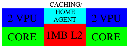
Figure 3: Schematic of a tile within a KNL processor.
