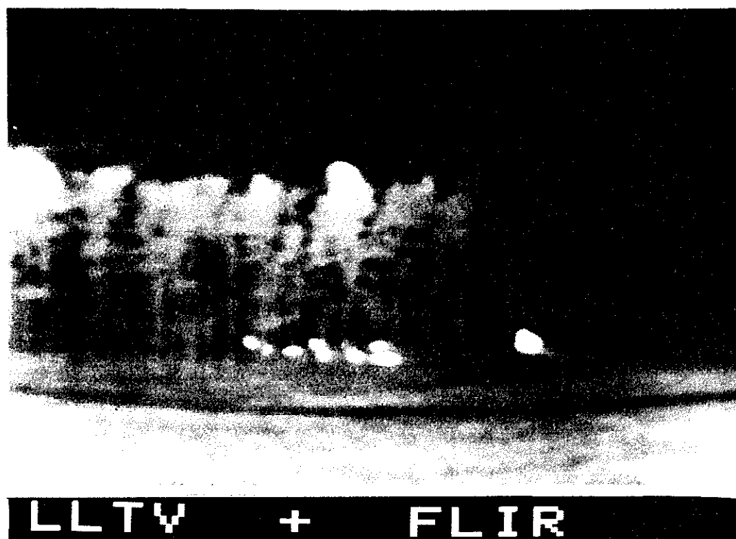
Fig 8 Computer generated combination of the same scene under visual and thermal conditions
