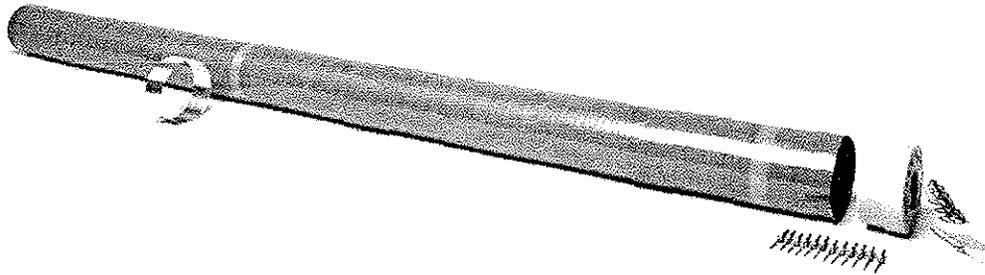
Figure 7.3 Supercritical shaft parts
