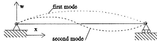
Figure 4.1 Shaft modelled as a hinged supported beam.
