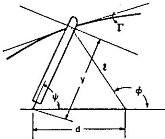
Fig. 3 Geometry of blade vortex intersection
