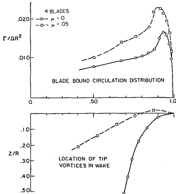
Fig. 12 Effect of cross flow on wake geometry at  $\mu = .05$  for a 4 bladed rotor
