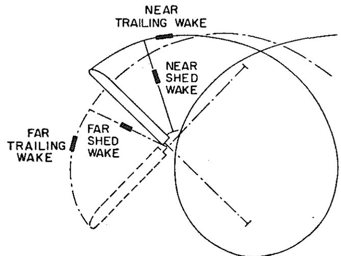
Fig. 1 Wake geometry showing near and far trailed and shed wakes
