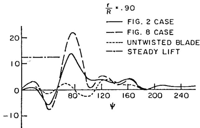
Fig. 9 Airloads due to wake interactions only vs. azimuth
