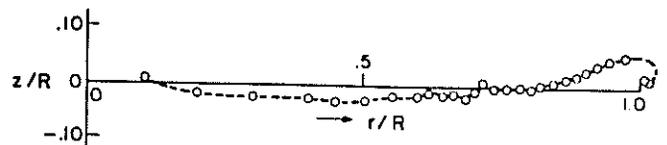
**Fig. 7** Roll up of near wake after  $\Delta\phi$  of  $90^\circ$  in forward flight ( $\mu = .39$ )
