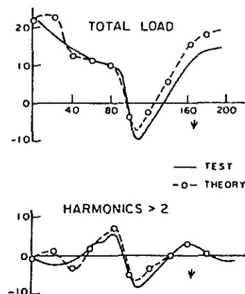
Fig. 8 Effects of wake distortion on airloads at 90% span
