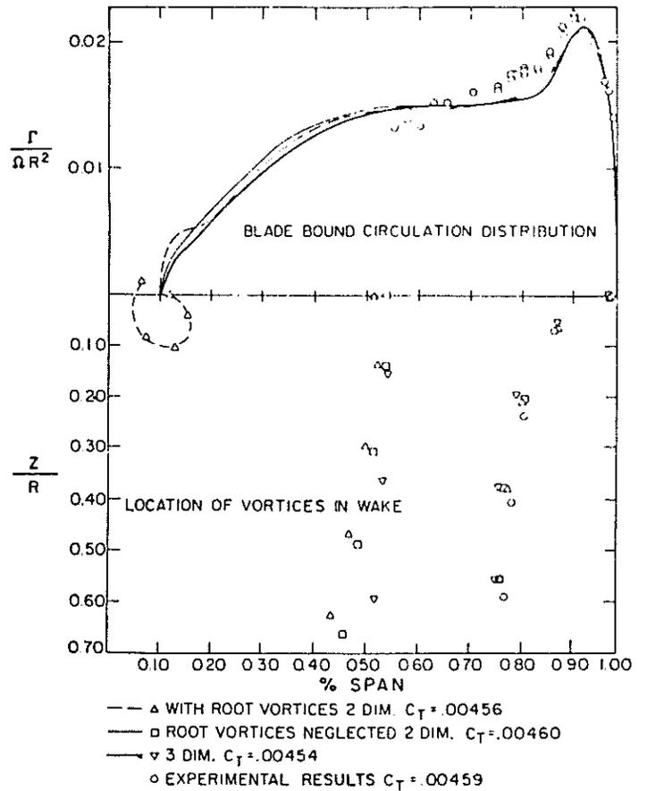
**Fig. 5** Blade bound vortex distribution and wake geometry in hover.
