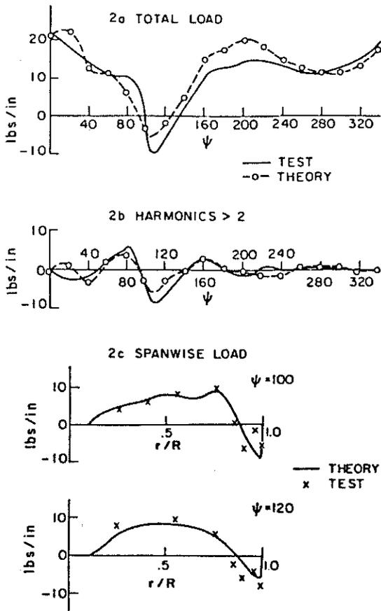
Fig. 2 Blade airloads at 90% span,  $\mu = .39$ . Experimental data from Ref. 5
