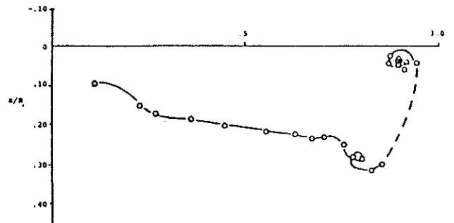
**Fig. 6** Roll up of wake from hovering rotor at  $\phi = 180^\circ$
