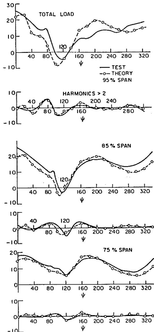
Fig. 4 Blade loads, total and with harmonics below 3rd removed, at various spanwise locations
