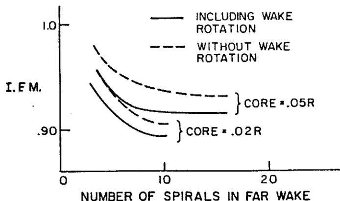
Fig. 11 Ideal figure of merit (IFM) in hover as a function of far wake modelling - 2 bladed rotor of Ref. 11
