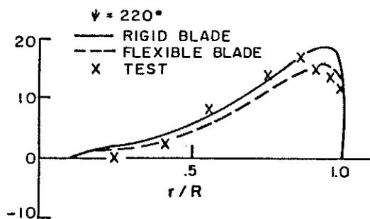
Fig. 10 Effect of higher harmonics of flapping and blade flexibility
