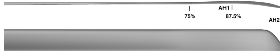
Figure 11: Top and side view of the optimal blade of the anhedral optimization
