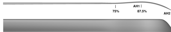
Figure 9: Top and side view of the optimal blade of the anhedral optimization
