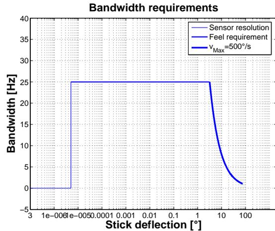
Fig 3 : Bandwidth requirements for the pitch/roll stick
