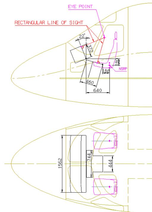
Fig 6 : Positioning of front-panel and interseat console.
