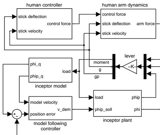
Fig 2 : Model following controller architecture (phi = Plant stick angle, phip = Plant stick angular velocity, phi\_q = Model stick angle, phip\_q = Model stick angular velocity, g = Deflection at FRP, gp = Velocity at FRP, v\_dem = Demanded velocity)
