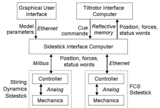
Fig 10: Control architecture
