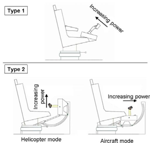
Fig 11: Two types of power inceptors
