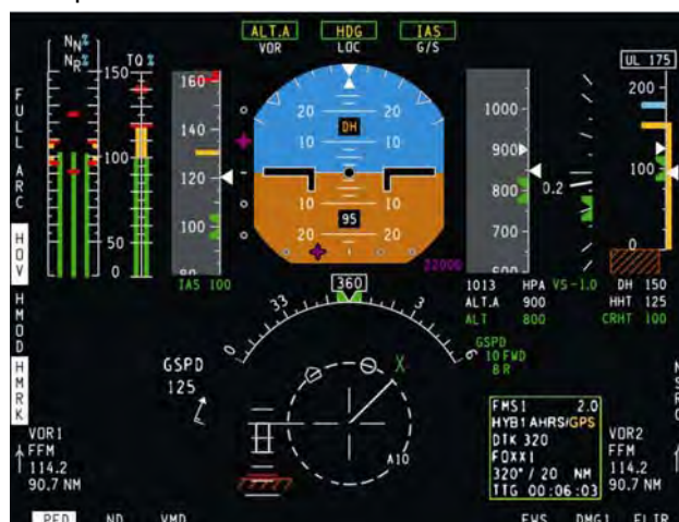
Figure 17: GAMS Primary Flight Display with Hover Page below the Attitude Direction Indicator
