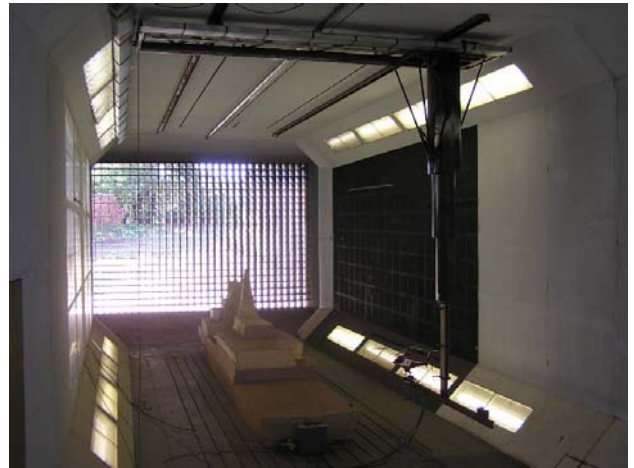
Figure 4 Wind tunnel setup of ~1:10 scale helicopter-ship interface
