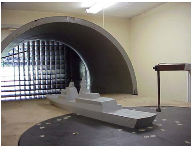
Figure 2 Higher fidelity 1:100 MEKO Class Frigate in 2mWT for flow field characterisation
