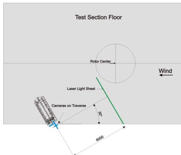
Figure 3 Location of measurement plane
