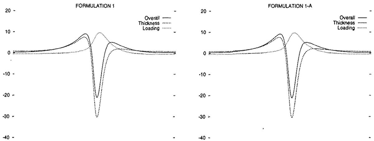
Figure 3 - Comparison between HERNOP acoustic pressure signatures, calculated by Farassat formulations 1 and 1-A, for an hovering rotor.
