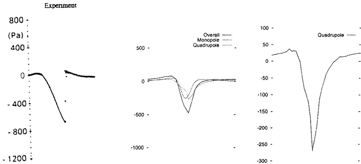
Figure 9 - HERNOP results for nonlifting, hovering rotor, at  $M_{tip}$  equal to 0.9. The flow field description given by aerodynamic input succeeds in breaking the symmetrical shape of quadrupole signature, but the resulting acoustic pressure is undervalued, with respect to the experimental results.
