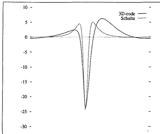
Figure 7 - Comparison between the predicted quadrupole noise signatures, from Schultz method and the volume integration (3D-code); the example refers to an hovering rotor at  $M_{tip} = 0.8$  and an observer position with  $r/R = 3.09$ .
