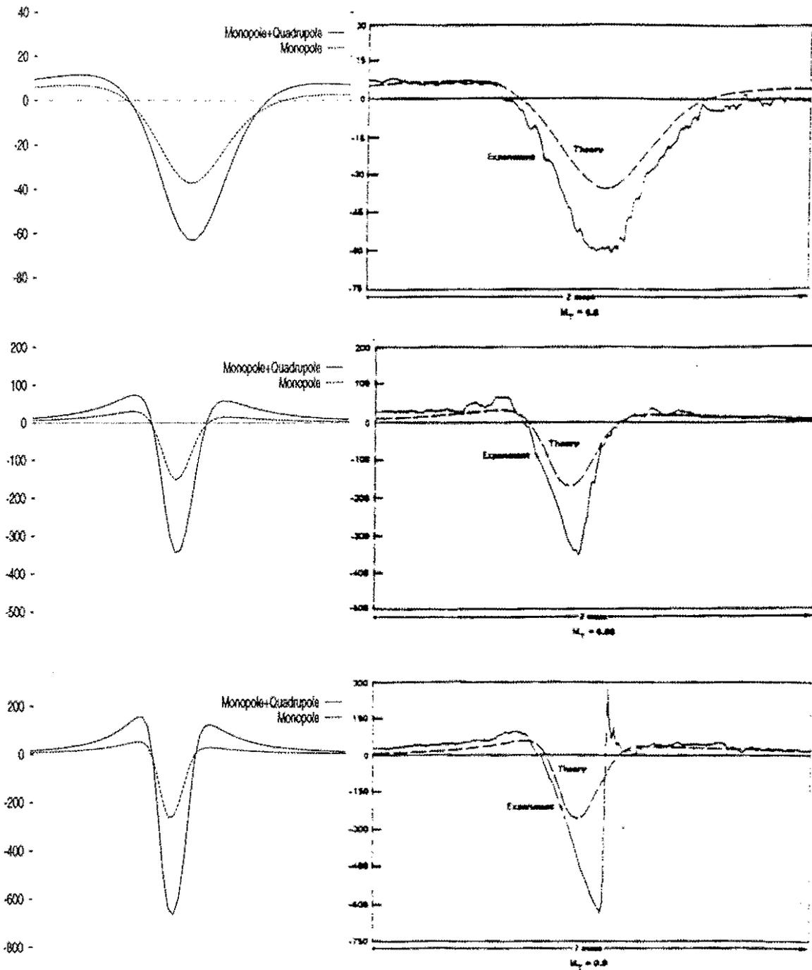
Figure 5 - Comparison of HERNOP predicted acoustic signatures with experimental pressure time histories, in-plane,  $r/D = 1.5$ ,  $M_{t,p} = 0.8, 0.88$  and  $0.9$ . The figures on the right have been extracted from [8]; the notation Theory refers to only monopole term calculation.
