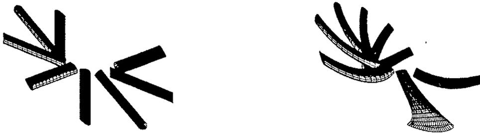
Figure 1 - Plot of eight successive positions of a rotor blade in forward flight and the corresponding retarded surface, as calculated by HERNOP.
