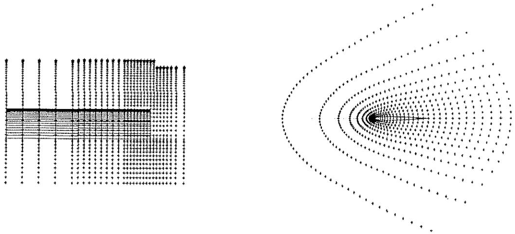
Figure 6 - Planform and side view of UTAH mesh for HERNOP validation tests.
