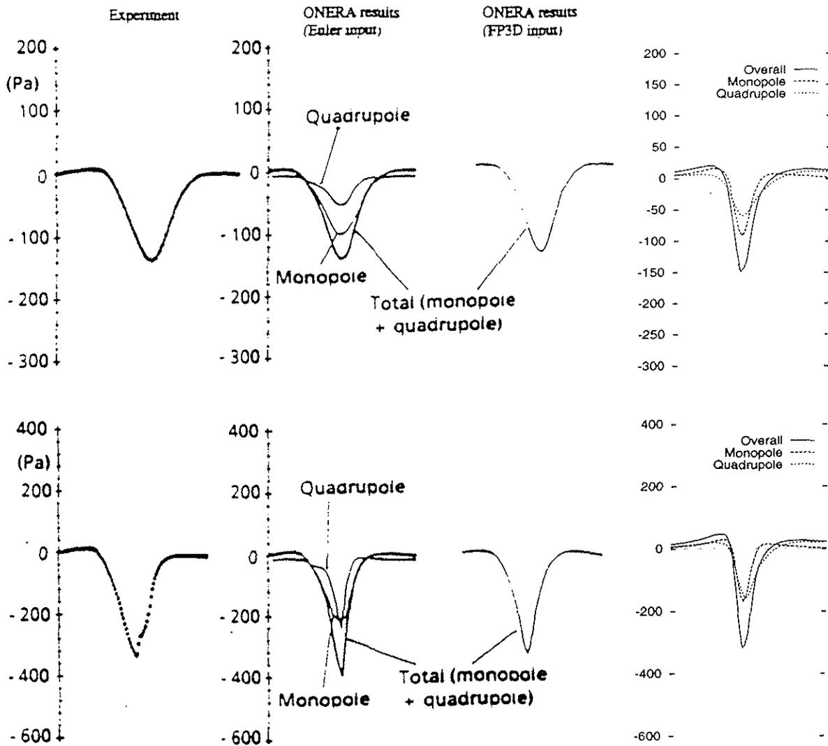
Figure 8 - Results for nonlifting, hovering rotor, at  $M_{tip}$  equal to 0.85, 0.88 are reported on the right. The observer position is at  $r/R = 3.09$
