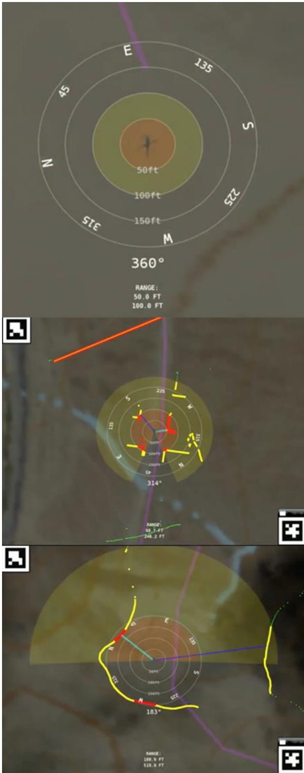
Figure 8. ICAD. Top: speed \leq 6 knots: 360° sweep extent, fixed-distance safety margin indicators, yellow Caution 75 ft. from blades, red Warning 25 ft. from blades. Center and Bottom: Speed \leq 6 knots: sweep extent decreases as speed increases, TTC-based safety margin indicators where ring radii increase as a function of speed, Caution 7.5 s from blades, Warning 2.5 s from blades.
