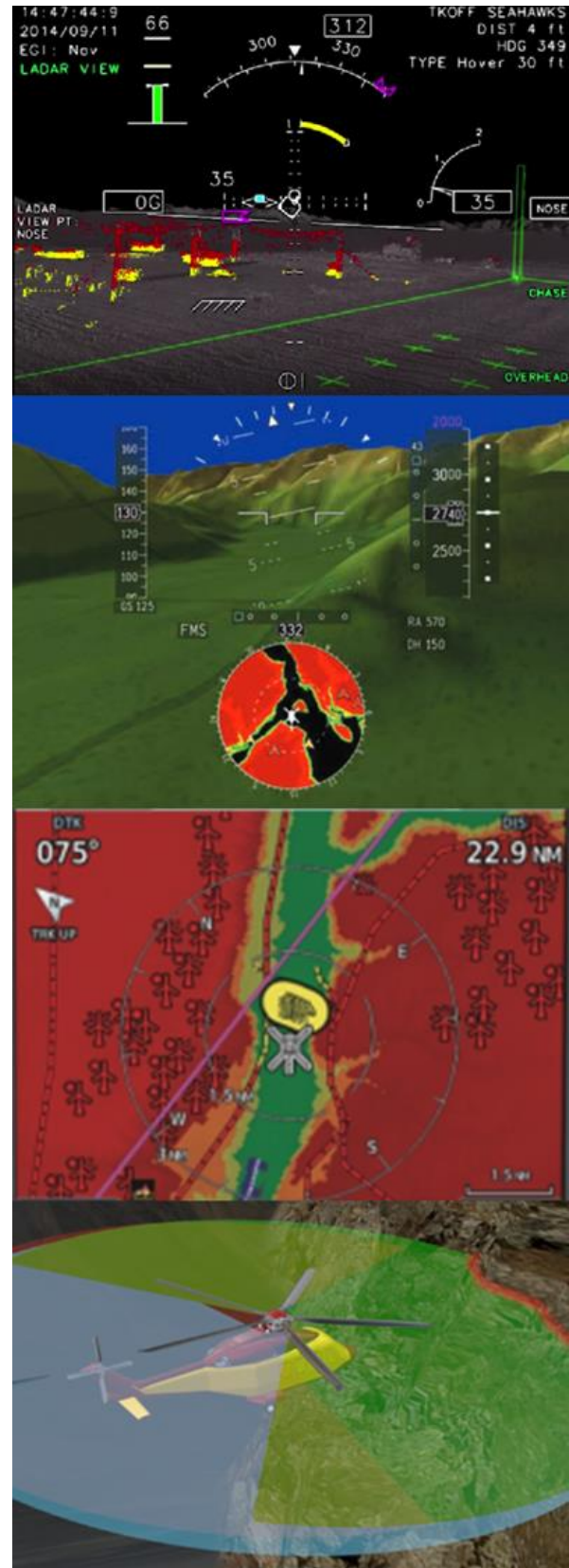
Figure 1. From top to bottom: EVS: ADD LADAR, SVS: Rockwell Collins, Garmin (with WireAware power line avoidance), and Augusta Westland OPLS.
