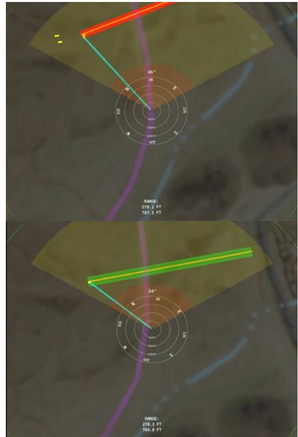
Figure 9. Power Line: clearance status is color-coded (red: ownship altitude below line, green: ownship altitude above line). The power line width expands outward from its nominal configuration at a 2Hz cycling rate to capture the pilot's attention. Note that this clearance behavior is not matched auditorily other than by the perception of elevation cues (above or below).
