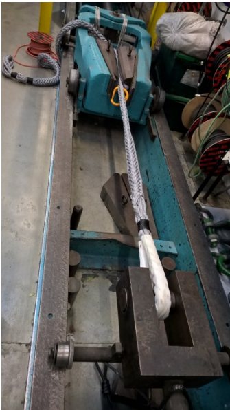
Figure 8: SPIE rope strength test
