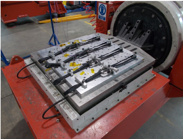
Figure 2: Vibration test connectors
