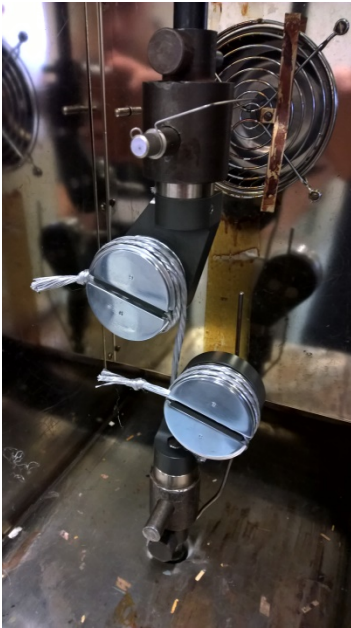
Figure 7: SPIE rope yarn strength test
