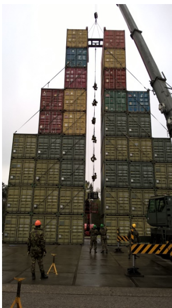
Figure 3: SPIE system drop test
