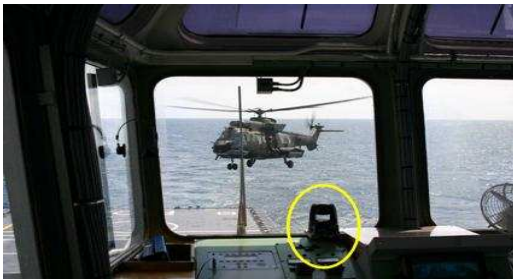
Figure 27. Video camera installed in the FLYCO cabinet.
