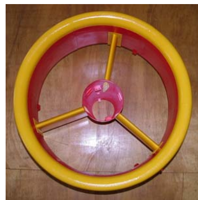
Fig. 20b : Duct and fuselage covered with polyurethane paint
