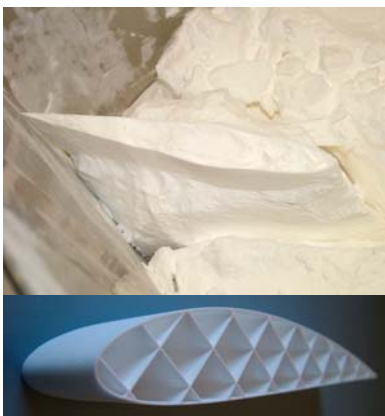
Fig. 22 : Lattice must allow excess of powder to be removed
