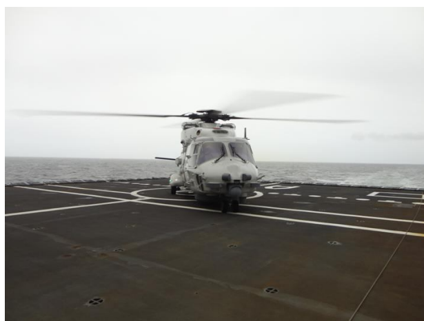
Figure 15; Missing 45° line on the deck
