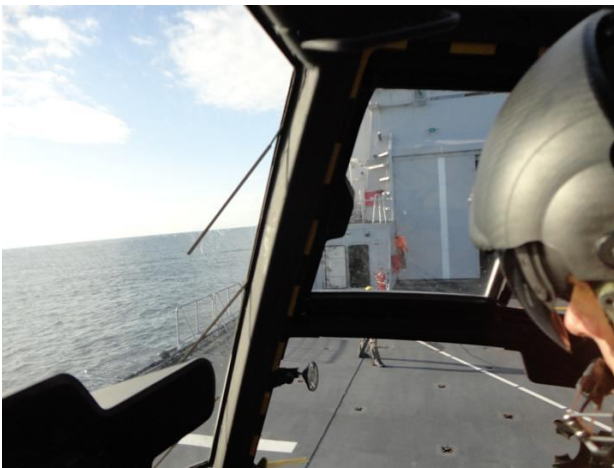
Figure 17; Obstruction horizontal bar in door
