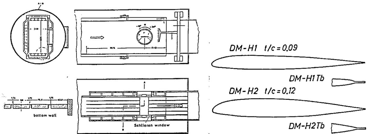
Fig. 6 Transonic Windtunnel Braunschweig (TWB) of DFVLR Fig. 7 Helicopter rotor blade airfoils DM-H1 and DM-H2
