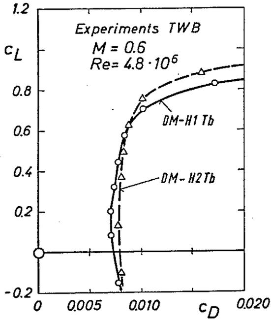
Fig. 12 Drag polars of the airfoils DM-H1 Tb and DM-H2 Tb
