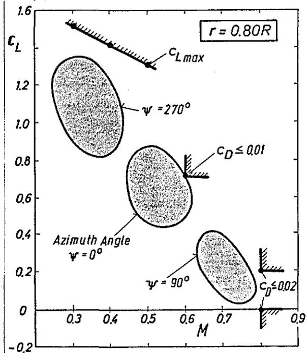
Fig. 5 Design objectives for the airfoil for the inner blade parts
