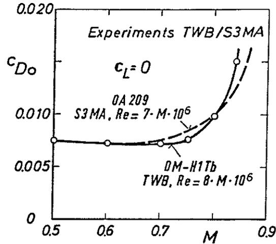
Fig. 14 Zero lift drag coefficients of several airfoils
