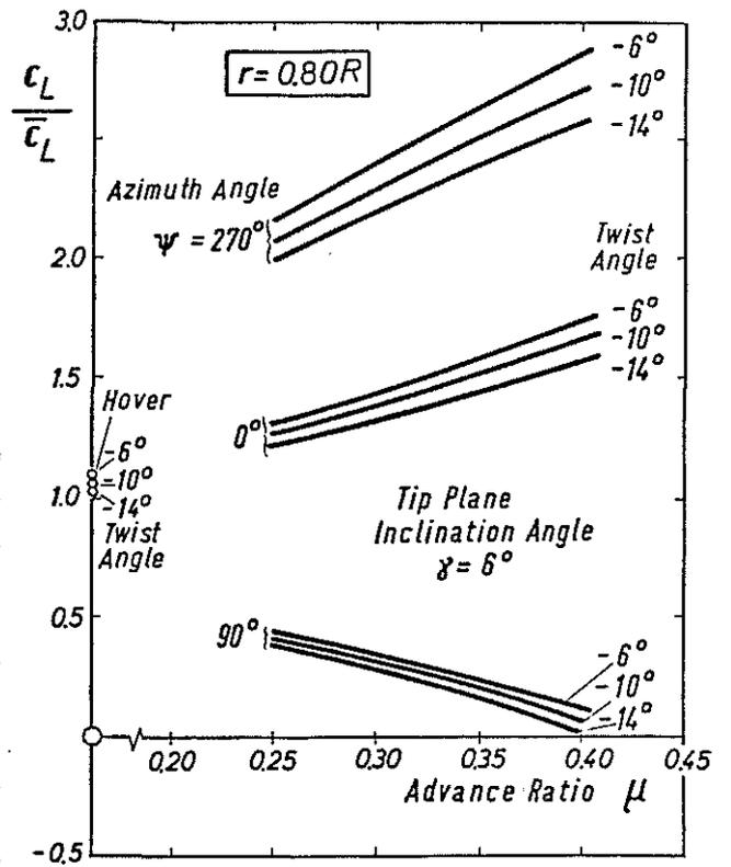
Fig. 3 Blade twist effect on blade lift coefficient for radial positions of 0.95 and 0.8 R
