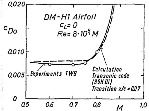
Fig. 21 Comparison of measured and calculated zero lift drag coefficients of the airfoil DM-H1
