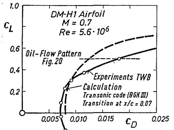
Fig. 19 Comparison of measured and calculated drag polars of the airfoil DM-H1 at  $M = 0.7$
