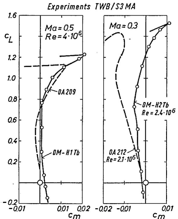
Fig. 16 Comparison of pitching moment coefficient evolution of several airfoils
