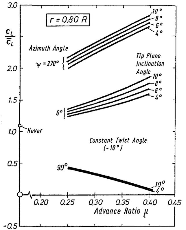
Fig. 2 Tip plane inclination effects on blade lift coefficient for radial positions of 0.95 and 0.8 R
