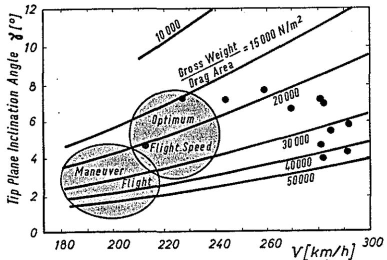
Fig. 1 Tip plane inclination angles of different helicopter types at maximum horizontal speed
