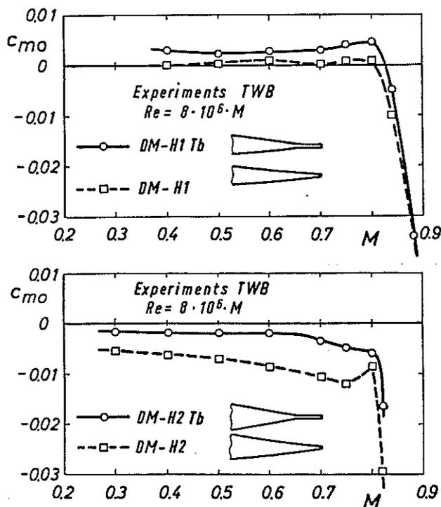
Fig. 10 Tab influence on zero lift pitching moment coefficient
