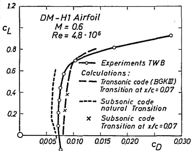
Fig. 18 Comparison of measured and calculated drag polars of the airfoil DM-H1 at  $M = 0.6$
