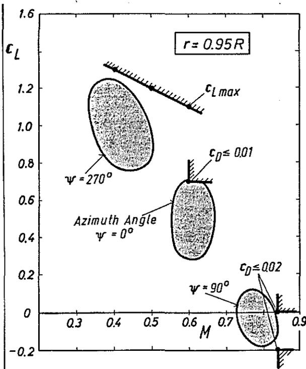
Fig. 4 Design objectives for the tip airfoil
