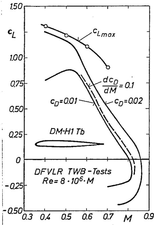
Fig. 8 Measured performance boundaries of the airfoil DM-H1 Tb
