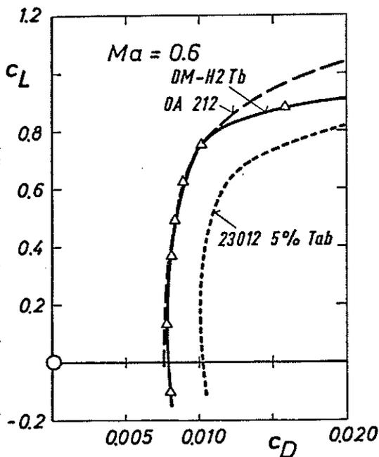
Fig. 13 Drag polars of several airfoils at M = 0.6
