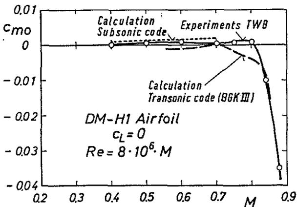
Fig. 22 Comparison of measured and calculated zero lift pitching moment coefficients of the airfoil DM-H1
