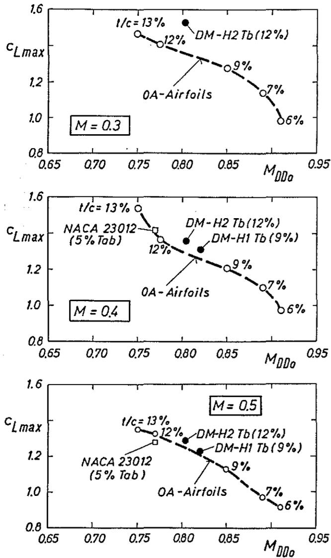
Fig. 17 Measured maximum lift coefficients and drag divergence Mach number of several rotor blade airfoils
