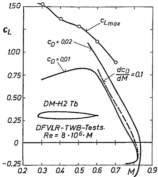
Fig. 9 Measured performance boundaries of the airfoil DM-H2 Tb
