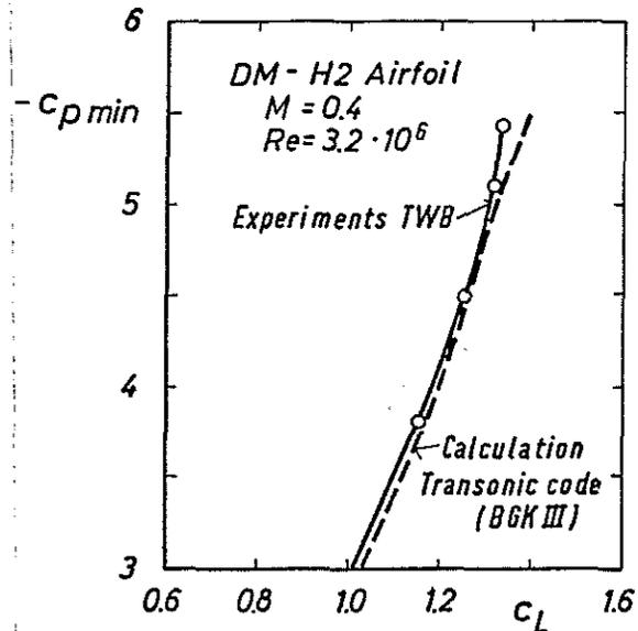
Fig. 23 Comparison of measured and calculated minimum pressure coefficient of the airfoil DM-H2
