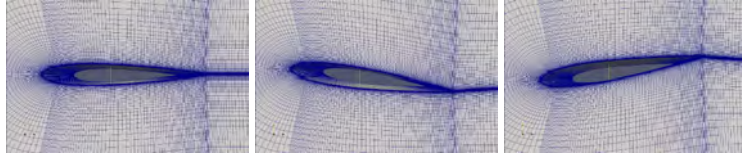
Figure 4: Computational mesh at various times in one of the dynamic stall cases
