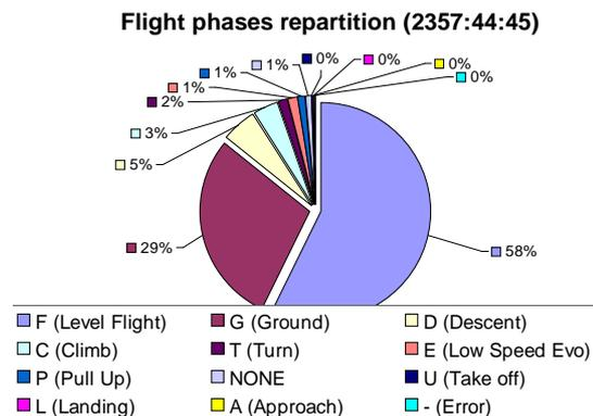
Figure 8. Flight spectrum
