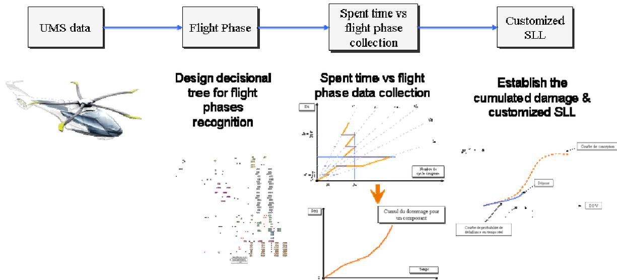
Figure 1. Service Life Limit calculation chain
