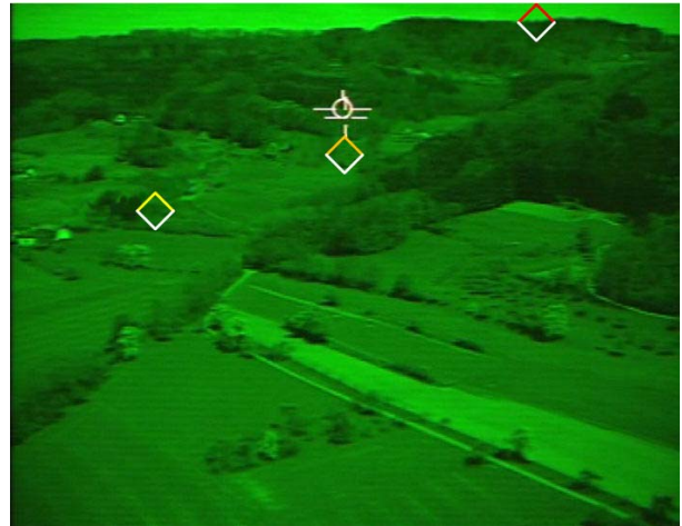
Figure 6 - CFIT WARNING WITH RISING DIAMONDS FOR A RISING TERRAIN WHERE THE HELICOPTER GETS CLOSE TO THE PREDEFINED SAFETY MARGIN OF 300 FT AGL STRAIGHT AHEAD AND CANNOT TURN RIGHT WITHOUT VIOLATING THE SAFETY MARGIN.
