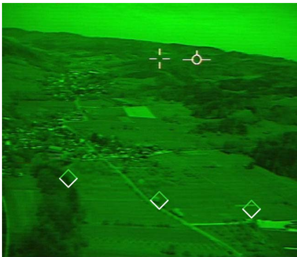
Figure 5 - CFIT WARNING WITH RISING DIAMONDS FOR A CASE SUFFICIENTLY ABOVE THE PREDEFINED SAFETY MARGIN OF 300 FT AGL.
