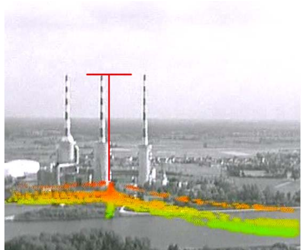
Figure 3 - APPROACH TO A POWER PLANT WITH DETECTED POWER LINE IN THE FOREGROUND AND SMOKE PIPES STILL OUT OF RANGE BUT IN THE ODB DISPLAYED AS A SINGLE OBSTACLE SYMBOL.
