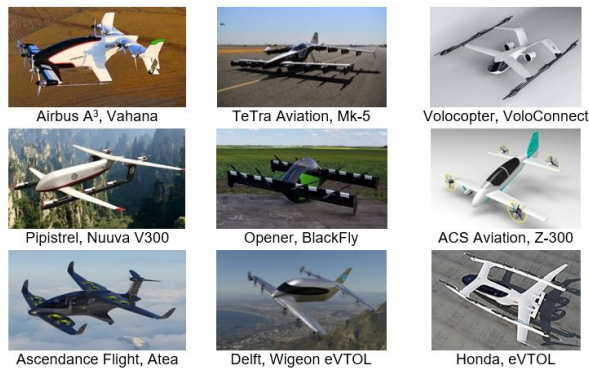
Figure 1 Notable Tandem Wing eVTOL Aircraft [3]–[11]
