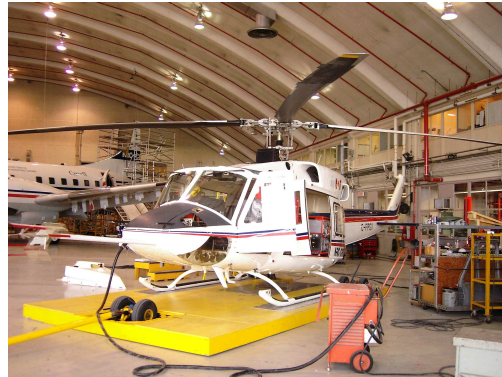
Figure 1.2: Bell 412 Advanced Systems Research Aircraft (ASRA), operated by NRC Canada
