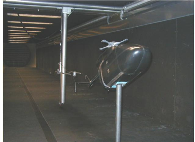
Fig. 5: Velocity measurement setup
